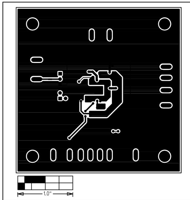
Figure 4. MAX1702 EV Kit PC Layout—Solder Side
