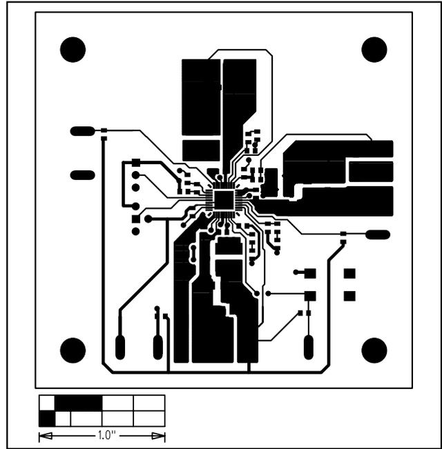
Figure 3. MAX1702 EV Kit PC Board Layout—Component Side
