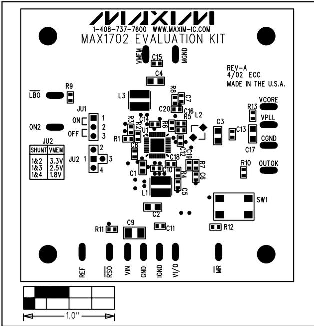
Figure 2. MAX1702 EV Kit Component Placement Guide—Component Side
