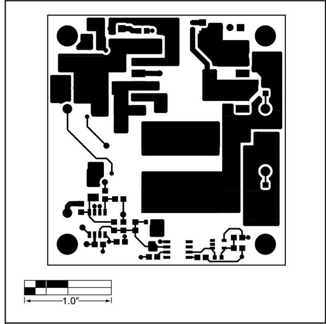
Figure 6. MAX5015 EV Kit PC Board Layout—Component Side
