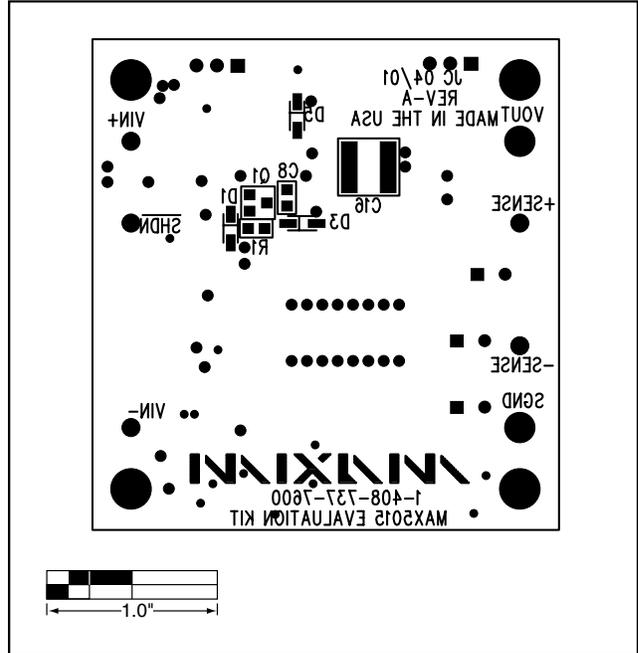
Figure 10. MAX5015 EV Kit Component Placement Guide—Solder Side
