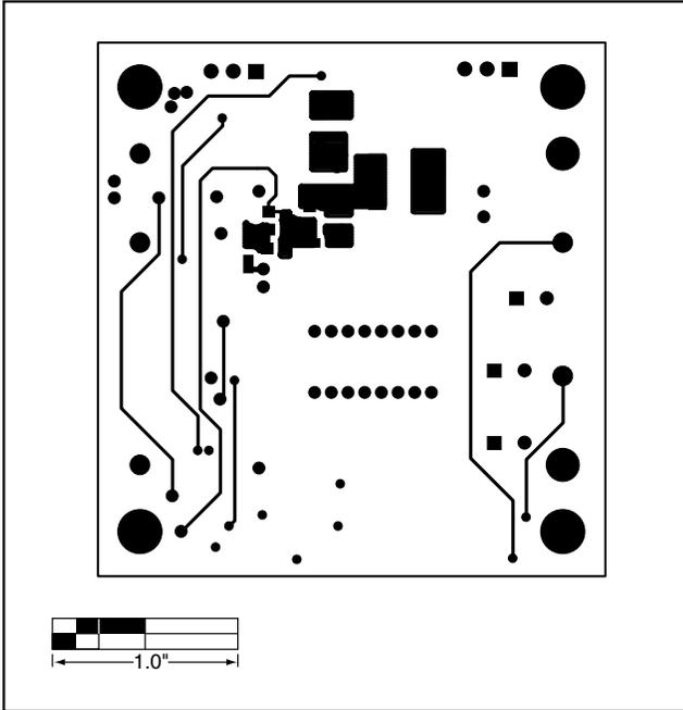
Figure 9. MAX5015 EV Kit PC Board Layout—Solder Side
