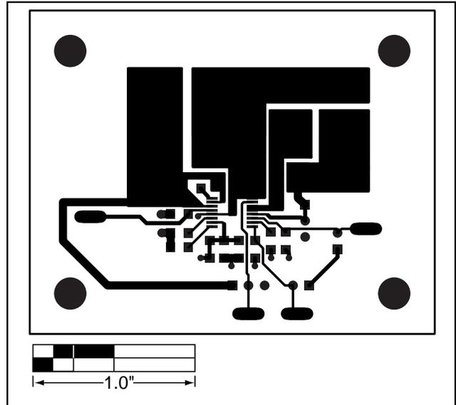
Figure 3. MAX1685 EV Kit PC Board Layout—Component Side
