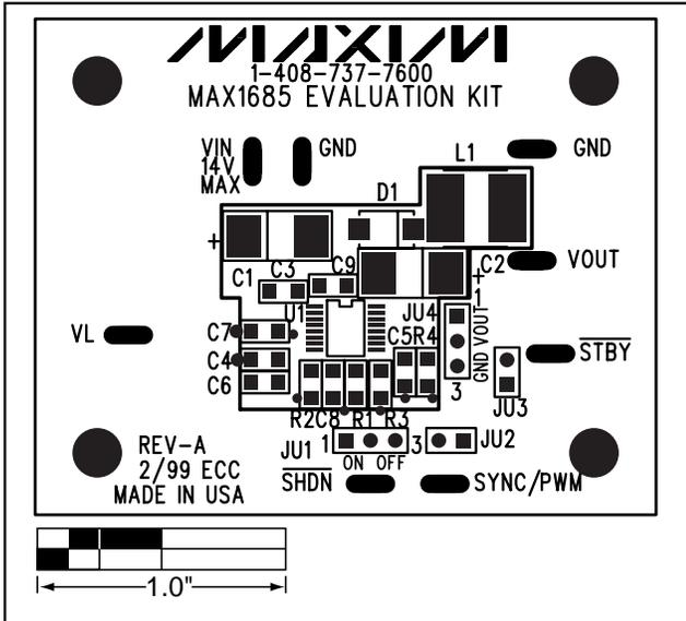
Figure 2. MAX1685 EV Kit Component Placement Guide—Component Side
