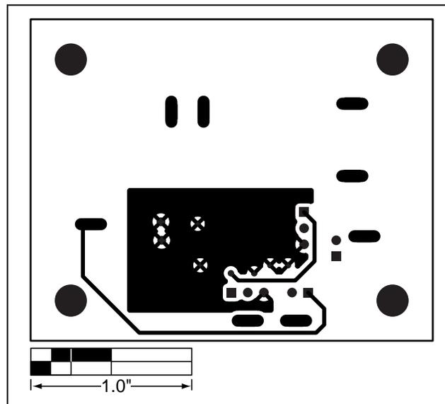
Figure 4. MAX1685 EV Kit PC Board Layout—Solder Side
