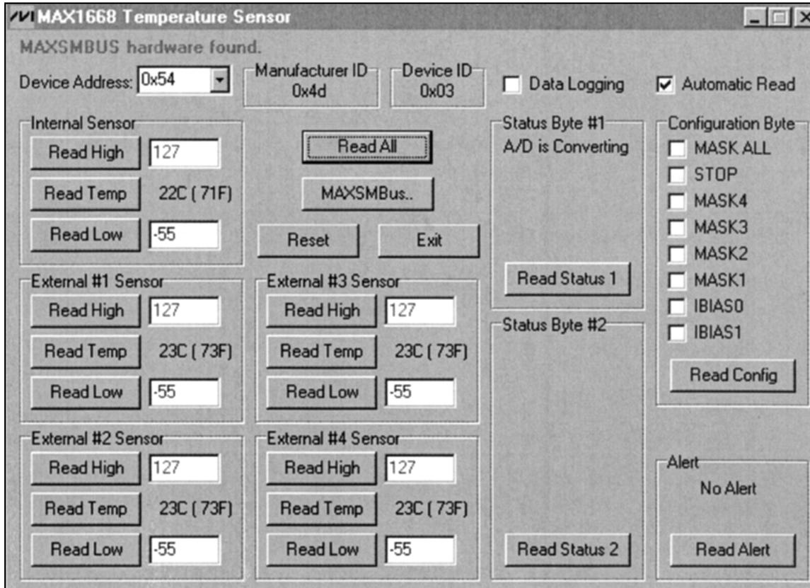
Figure 1. Main Display for MAX1668 EV Kit
