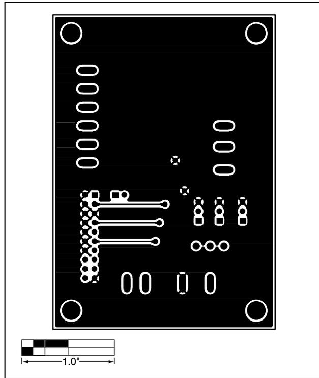
Figure 5. MAX1668 EV Kit PC Board layout—Solder Side
