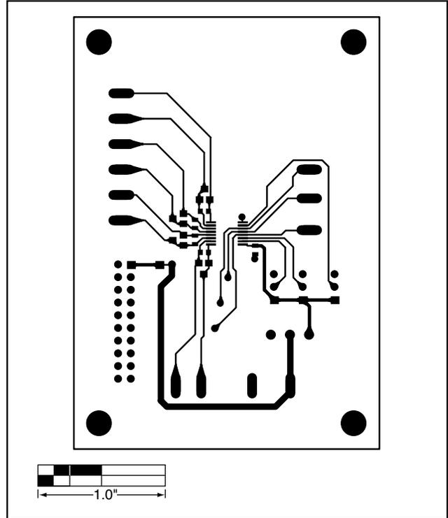
Figure 4. MAX1668 EV Kit PC Board Layout—Component Side
