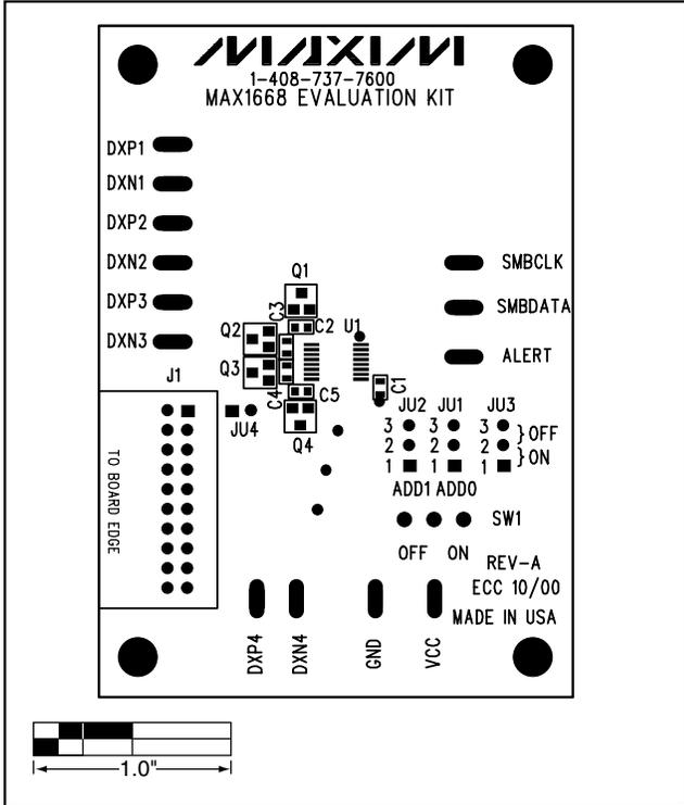
Figure 3. MAX1668 EV Kit Component Placement Guide—Component Side
