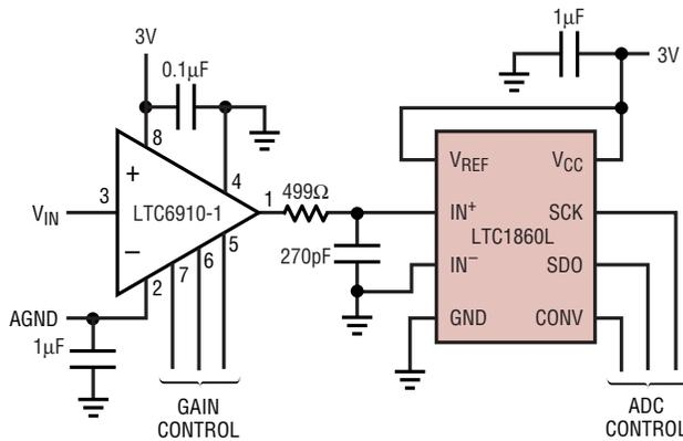
LTC6910-1 (IN TSOT-23 PACKAGE) COMPACTLY ADDS 40dB OF INPUT GAIN RANGE TO THE LTC1860L (IN MSOP 8-PIN PACKAGE). SINGLE 3V SUPPLY
