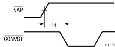
**Figure 9. NAP to CONVST Wake-Up Timing**
