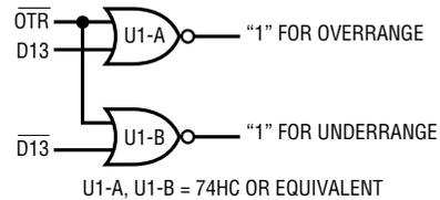
**Figure 8. Overage and Underrange Logic**
