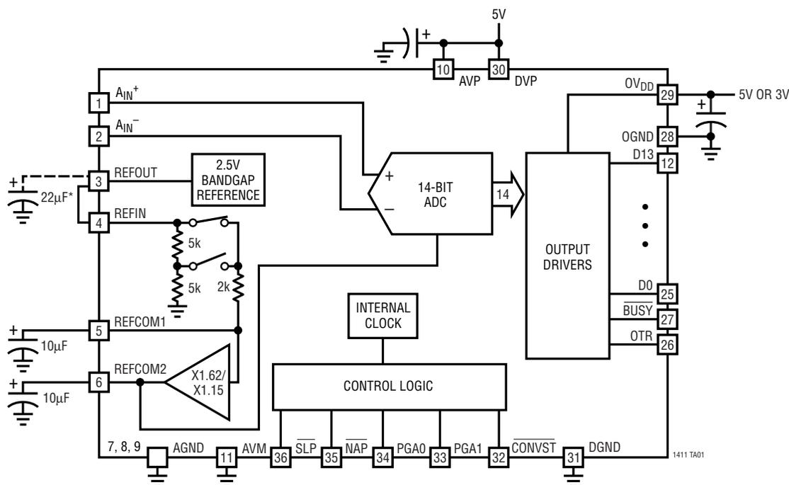
\*A 22 $\mu$ F CAPACITOR IS NEEDED IF REFOUT IS USED TO DRIVE  $A_{IN-}$
