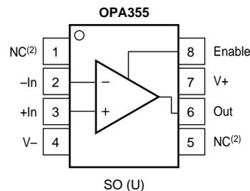
NOTES: (1) Pin 1 of the SOT23-6 is determined by orienting the package marking as indicated in the diagram. (2) NC indicates no internal connection.
