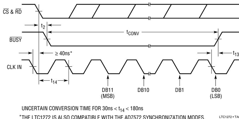
Figure 5.  $\overline{\text{RD}}$  and CLK IN for Synchronous Operation
