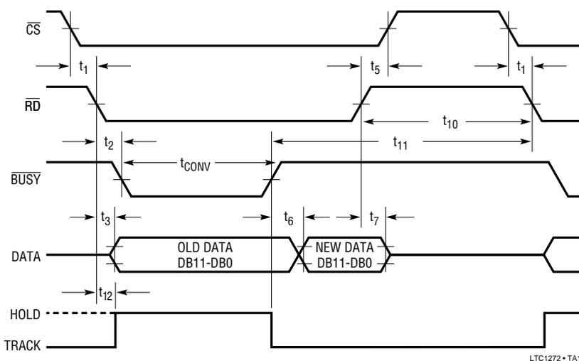
Figure 14. Slow Memory Mode, Parallel Read Timing Diagram
