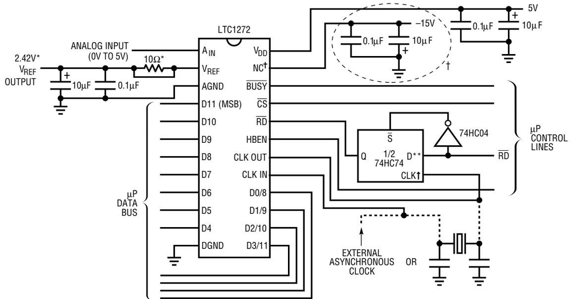
\* THE LTC1272 HAS THE SAME 0V TO 5V INPUT RANGE BUT PROVIDES A 2.42V REFERENCE OUTPUT AS OPPOSED TO THE -5.25V OF THE AD7572. FOR PROPER OPERATION, REVERSE THE REFERENCE CAPACITOR POLARITY AND SHORT OUT THE 10Ω RESISTOR.
