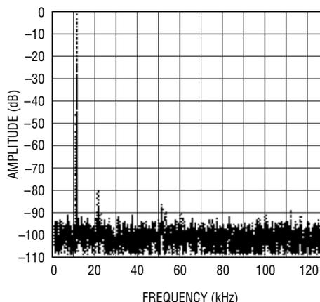
Figure 2. LTC1272 Non-Averaged, 1024 Point FFT Plot.
