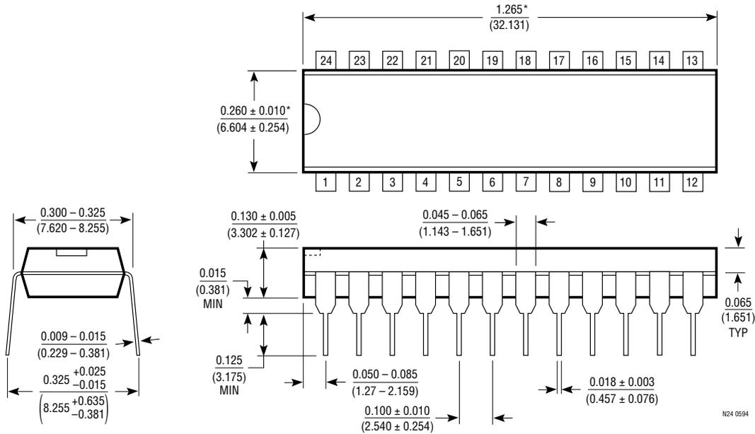
\*THESE DIMENSIONS DO NOT INCLUDE MOLD FLASH OR PROTRUSIONS. MOLD FLASH OR PROTURSIONS SHALL NOT EXCEED 0.010 INCH (0.254mm).
