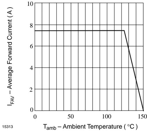
Figure 1. Max. Average Forward Current vs. Ambient Temperature
