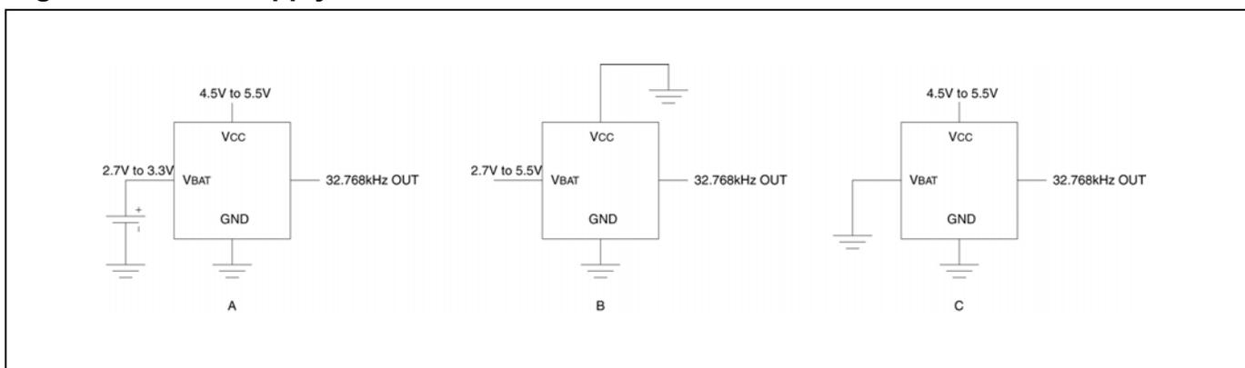
Figure 5 illustrates how a standard 32.768kHz crystal and the DS32kHz should be connected to address the interchangeable option. Using this connection scheme and the recommended layout provides a solution, which requires no hardware modifications. Only one device should be used at a time, and both layouts should be located very close together if the recommended layout is not used.
