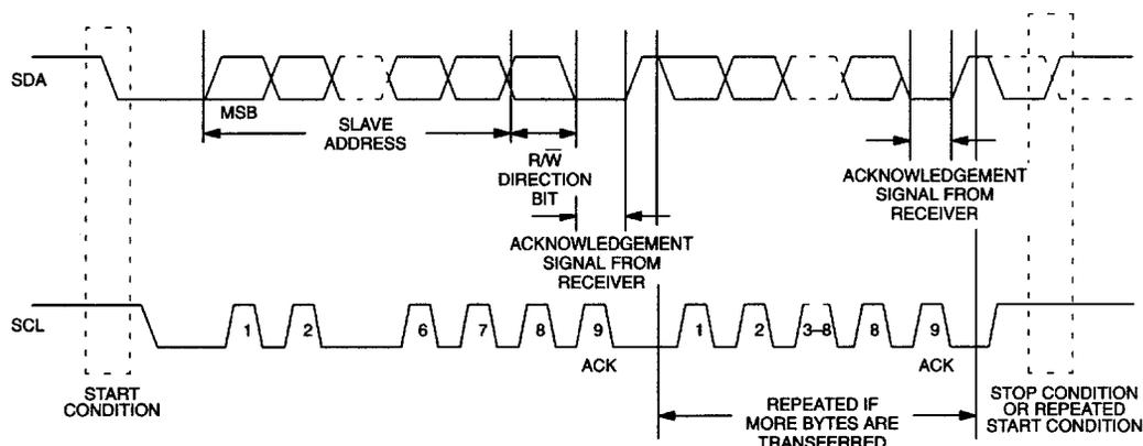
Figure 6 details how data transfer is accomplished on the two-wire bus. Depending upon the state of the  $R/\bar{W}$  bit, two types of data transfer are possible:
