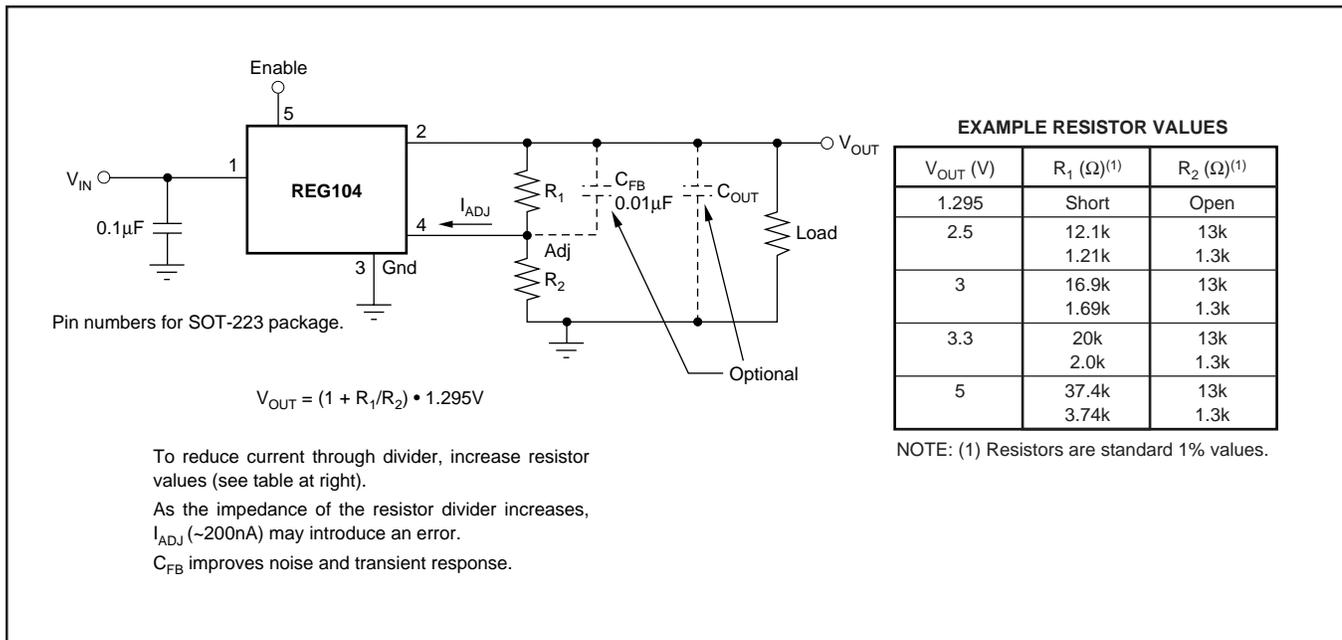
FIGURE 2. Adjustable Voltage Circuit for REG104A.
