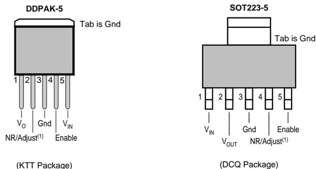
NOTE: (1) For REG104A-A: voltage setting resistor pin.
