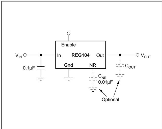
FIGURE 1. Fixed Voltage Nominal Circuit for REG104.
