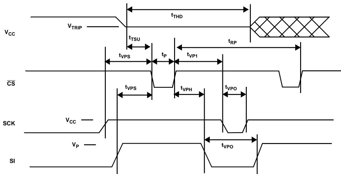
FIGURE 14.  $V_{TRIP}$  RESET CONDITIONS
