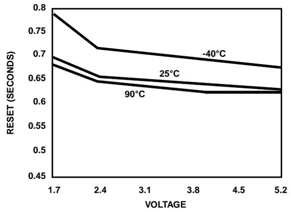
FIGURE 18.  $t_{WDO}$  VS. VOLTAGE/TEMPERATURE (WD1, 0 = 1, 0)
