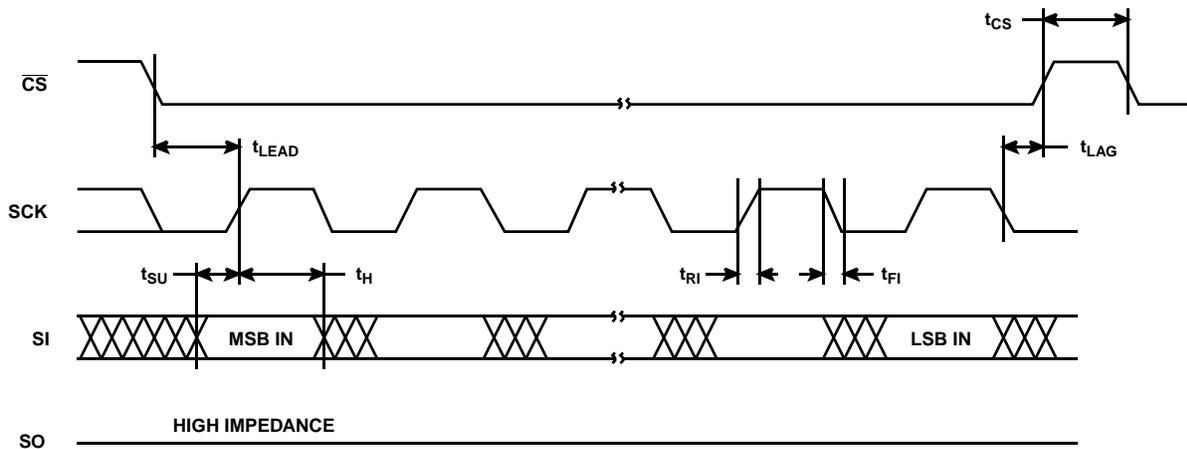
FIGURE 11. SERIAL INPUT TIMING
