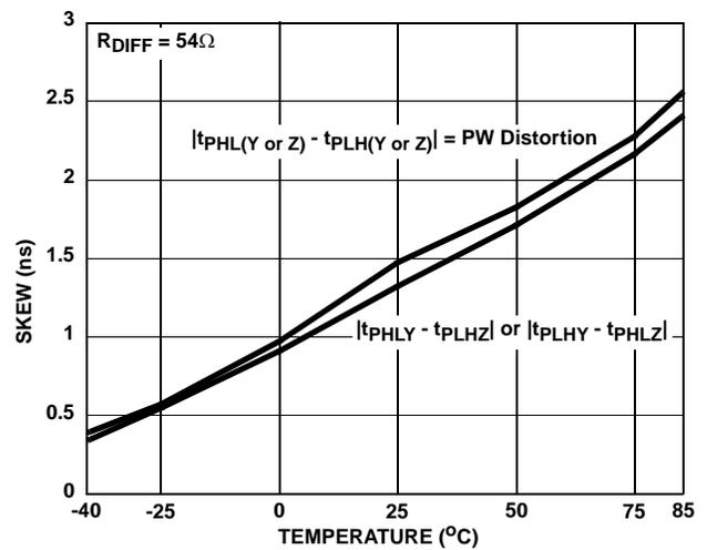
FIGURE 12. DRIVER SKEW AND PULSE DISTORTION vs TEMPERATURE
