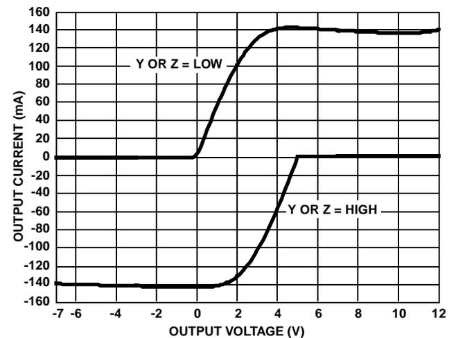
FIGURE 8. DRIVER OUTPUT CURRENT vs SHORT CIRCUIT VOLTAGE
