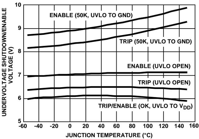
FIGURE 7. UNDERVOLTAGE THRESHOLD
