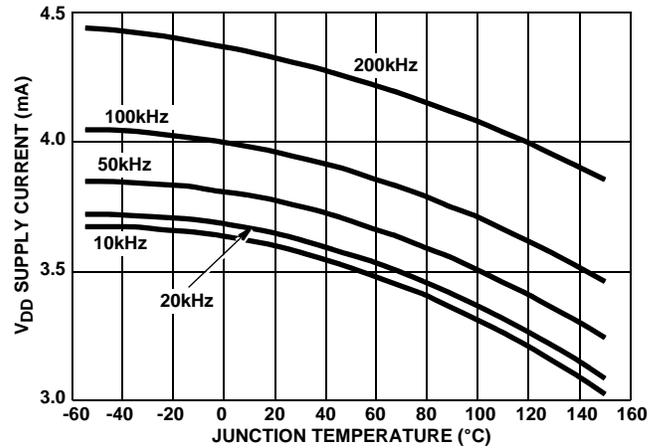
FIGURE 2.  $V_{DD}$  SUPPLY CURRENT vs SWITCHING FREQUENCY
