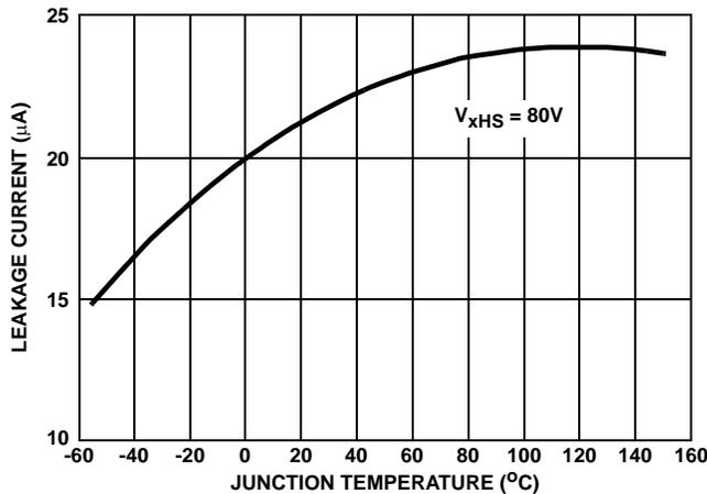
FIGURE 17. I<sub>xHS</sub> LEAKAGE CURRENT
