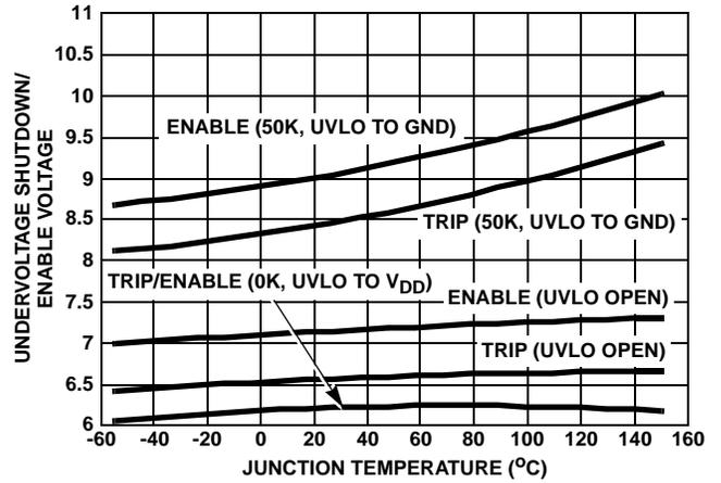
FIGURE 16. UNDERVOLTAGE THRESHOLD
