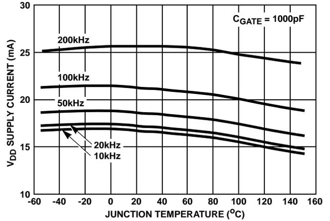
FIGURE 4.  $V_{DD}$  SUPPLY CURRENT vs SWITCHING FREQUENCY
