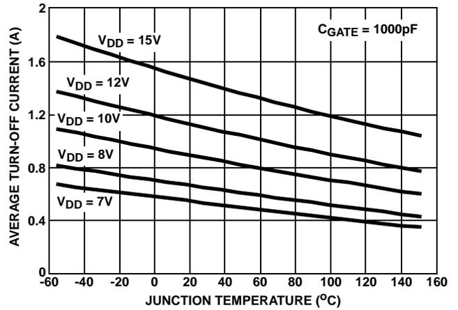
FIGURE 10. AVERAGE TURN-OFF CURRENT ( $V_{DD}$  TO 4V)
