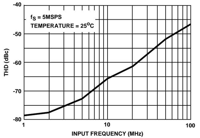
FIGURE 6. TOTAL HARMONIC DISTORTION (THD) vs INPUT FREQUENCY
