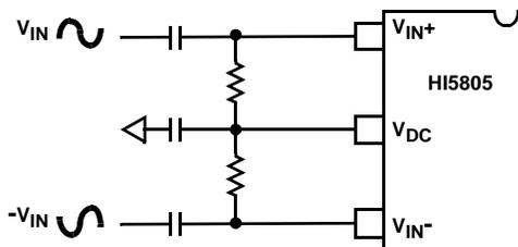
FIGURE 15. AC COUPLED DIFFERENTIAL INPUT
