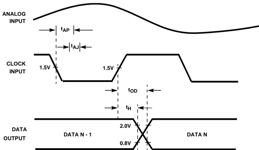
FIGURE 2. INPUT-TO-OUTPUT TIMING
