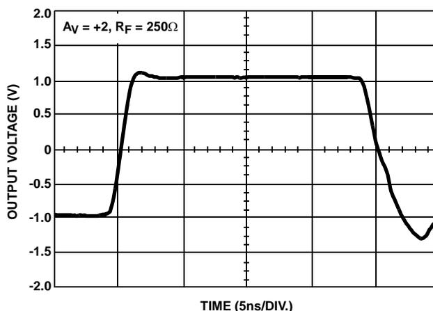
FIGURE 9. LARGE SIGNAL BIPOLAR PULSE RESPONSE
