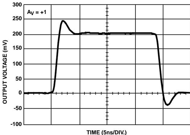
FIGURE 10. SMALL SIGNAL POSITIVE PULSE RESPONSE
