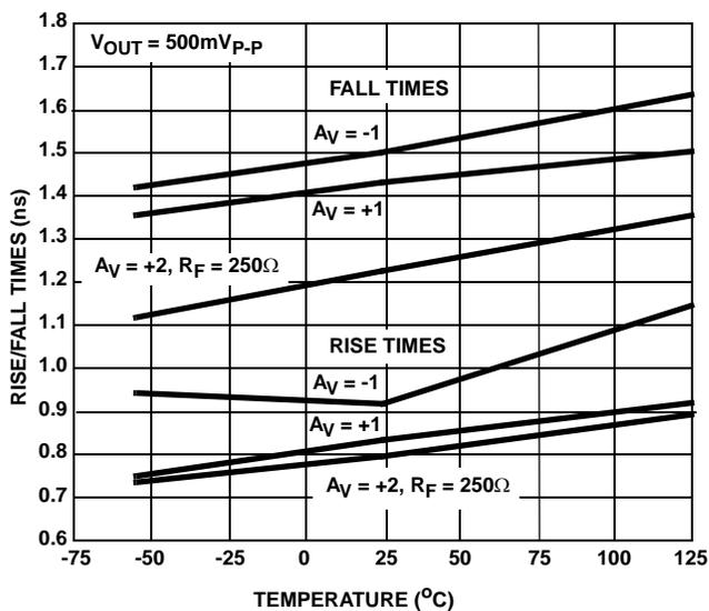
FIGURE 39. RISE AND FALL TIMES vs TEMPERATURE
