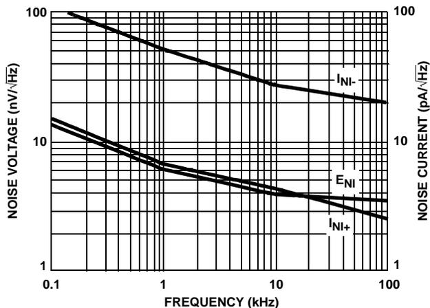
FIGURE 29. INPUT NOISE CHARACTERISTICS
