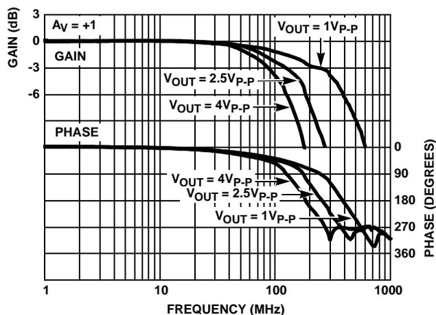
FIGURE 20. FREQUENCY RESPONSE FOR VARIOUS OUTPUT VOLTAGES
