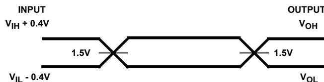
NOTE: Input test signals must switch between V<sub>IL</sub> (maximum) -0.4V and V<sub>IH</sub> (minimum) +0.4V.  $\overline{\text{RES}}$  and  $\overline{\text{F/C}}$  must switch between 0.4V and V<sub>CC</sub> -0.4V. Input rise and fall times driven at 1ns/V. V<sub>IL</sub> ≤ V<sub>IL</sub> (max) -0.4V for CSYNC pin. V<sub>CC</sub> -4.5V and 5.5V.
