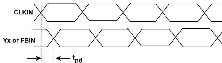
**Figure 2. Propagation Delay Time  $t_{pLH}$ ,  $t_{pHL}$**
