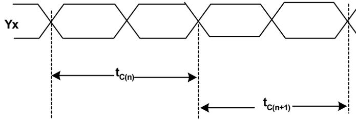
Figure 3. Cycle-to-cycle Jitter
