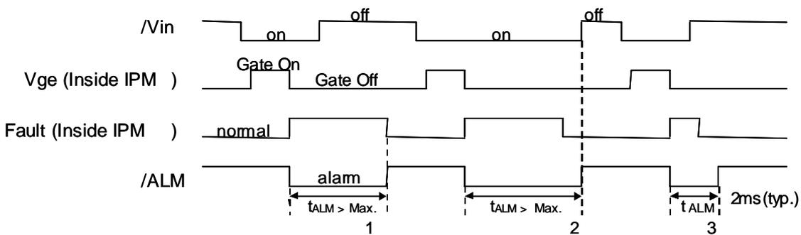
Fault : Over-current, Over-heat or Under-voltage
