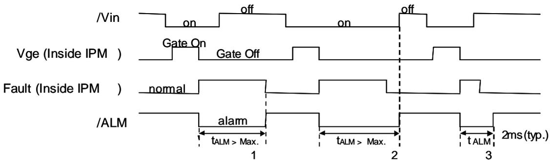
Fault : Over-current, Over-heat or Under-voltage
