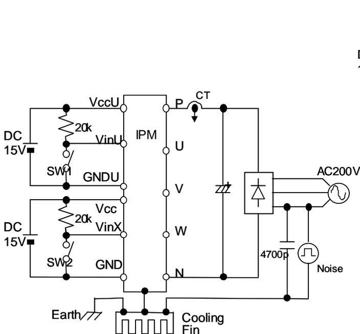
Figure 5. Noise Test Circuit
