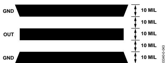
Figure 29. Use Separate Traces to Reduce Power Supply Noise
