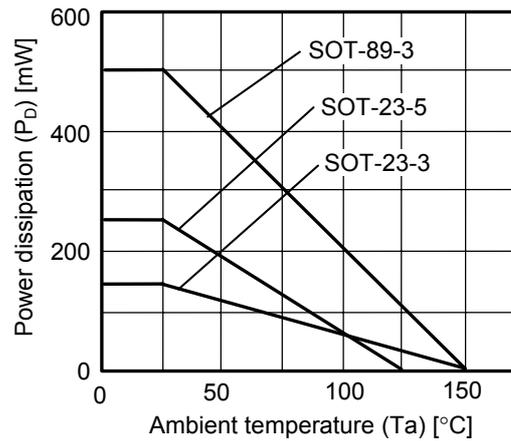
**Figure 7 Power Dissipation of The Packages (Before Mounting)**
