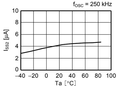
(3) Current Consumption at Shutdown ( $I_{SSS}$ ) vs. Temperature ( $T_a$ )
