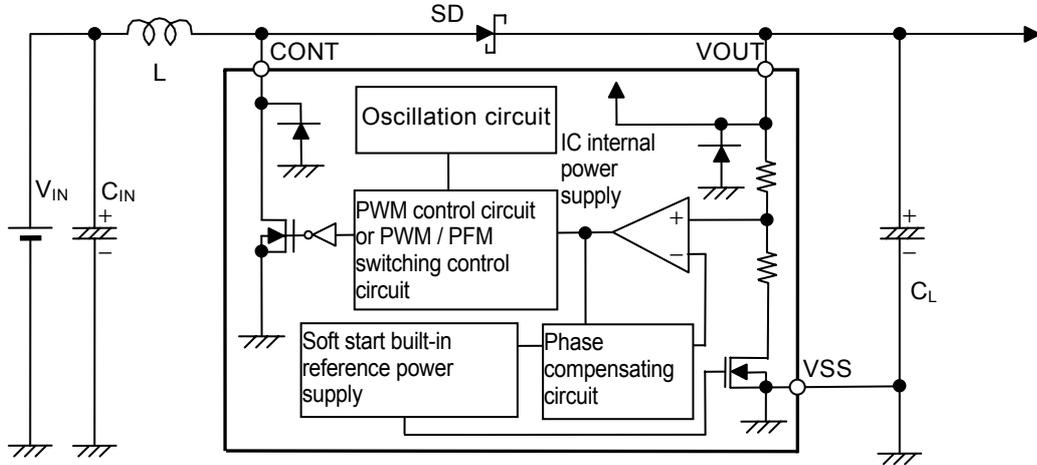
**Remark** The power supply for the IC chip is from the VOUT pin.
