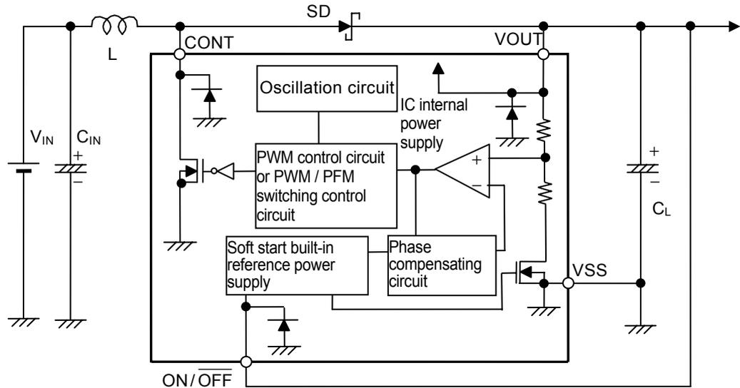
**Remark** The power supply for the IC chip is from the VOUT pin.
