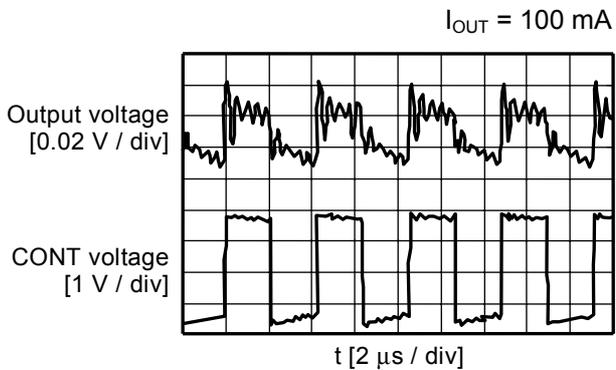
4. Examples of Transient Response Characteristics (Ta=25°C, 250 kHz, S-8354H33)
