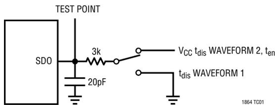
Voltage Waveforms for SDO Rise and Fall Times,  $t_r$ ,  $t_f$
