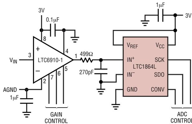
LTC6910-1 (IN TSOT-23 PACKAGE) COMPACTLY ADDS 40dB OF INPUT GAIN RANGE TO THE LTC1864L (IN MSOP 8-PIN PACKAGE). SINGLE 3V SUPPLY
