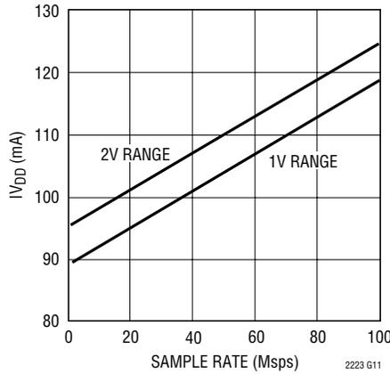
**LTC2223:  $I_{OVDD}$  vs Sample Rate, 5MHz Sine Wave Input,  $-1\text{dB}$ ,  $OV_{DD} = 1.8\text{V}$**
