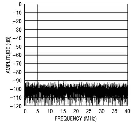
**LTC2222: 8192 Point FFT,  $f_{IN} = 30\text{MHz}$ ,  $-1\text{dB}$ , 2V Range**
