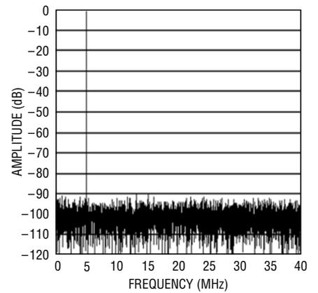
**LTC2223: 8192 Point FFT,  $f_{IN} = 30\text{MHz}$ ,  $-1\text{dB}$ , 2V Range**
