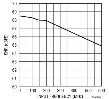
LTC2223: SNR vs Input Frequency, -1dB, 1V Range
