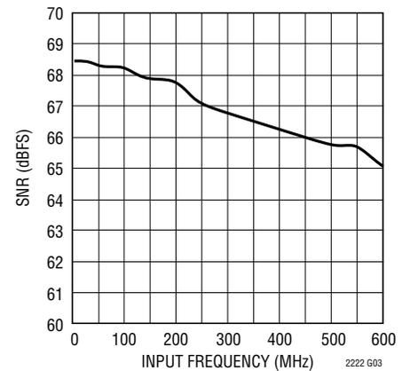
LTC2222: SNR vs Input Frequency, -1dB, 1V Range
