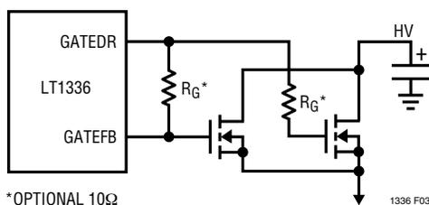
Figure 3. Paralleling MOSFETs
