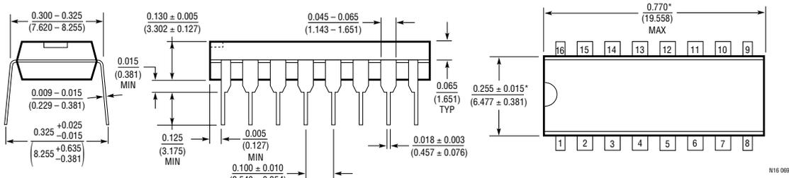
\*THESE DIMENSIONS DO NOT INCLUDE MOLD FLASH OR PROTRUSIONS.
