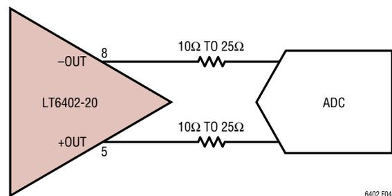
Figure 4. Adding Small Series R at LT6402 Output
