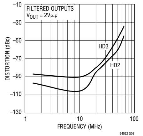
**Distortion vs Frequency, Differential Input, No  $R_{LOAD}$**
