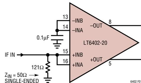
**Figure 1. Input Termination for Single-Ended 50 $\Omega$  Input Impedance**
