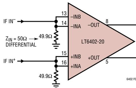
Figure 2. Input Termination for Differential 50Ω Input Impedance
