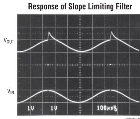
Figure 2. Lowpass Slope Limiting Filter with 0 TC
