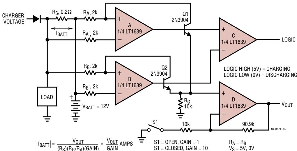
Figure 5. Battery Monitor
