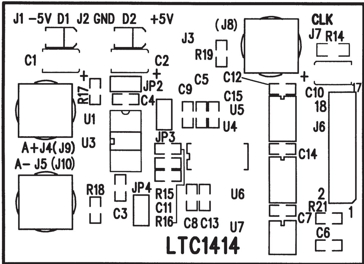
Figure 16b. Evaluation Circuit Board Component Side Silkscreen
