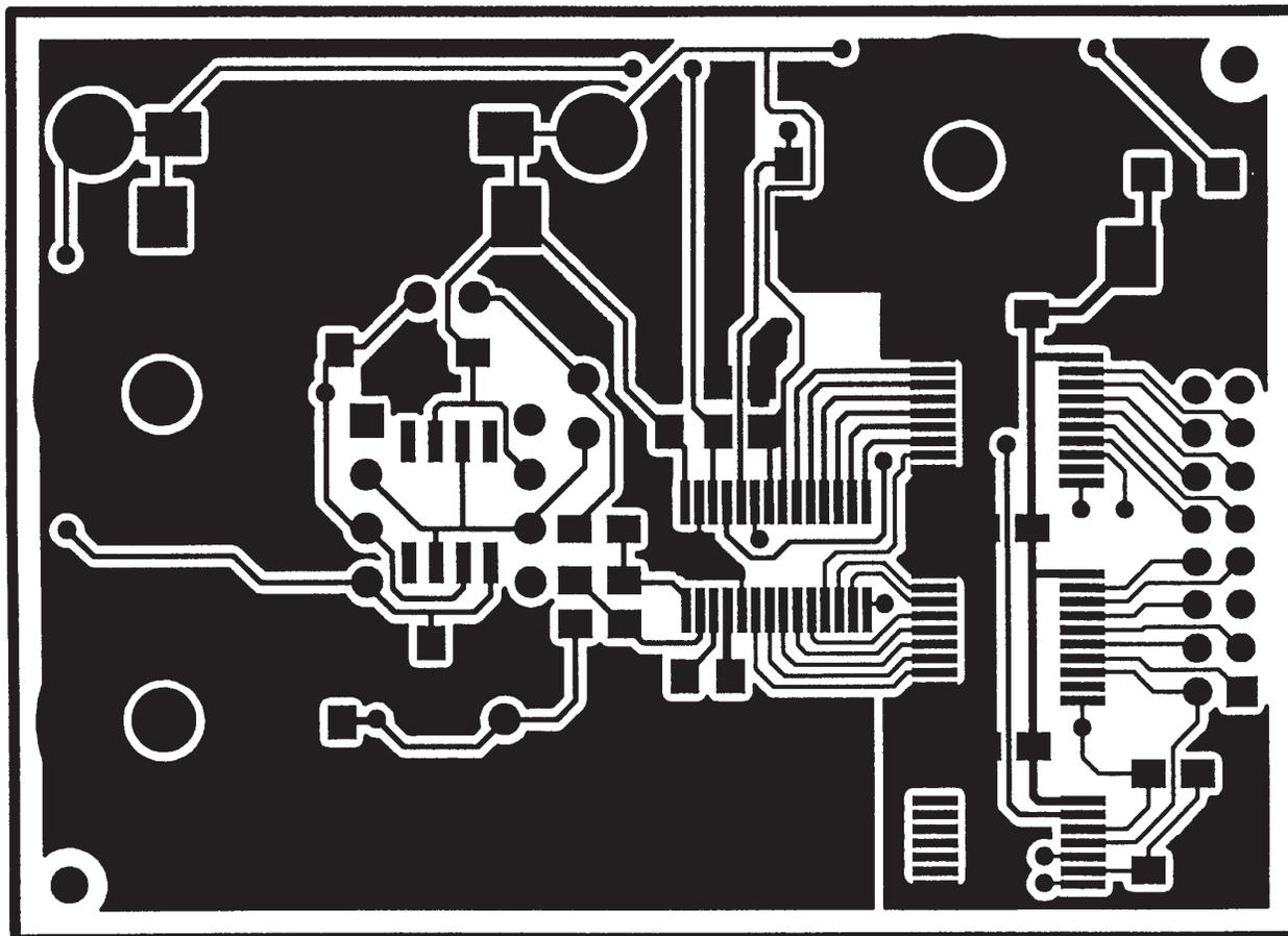
Figure 16c. Evaluation Circuit Board Component Side Layout
