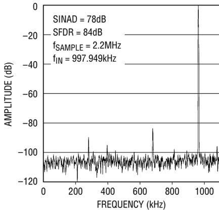
**Figure 2b. LTC1414 2048 Point FFT, Input Frequency = 1MHz**
