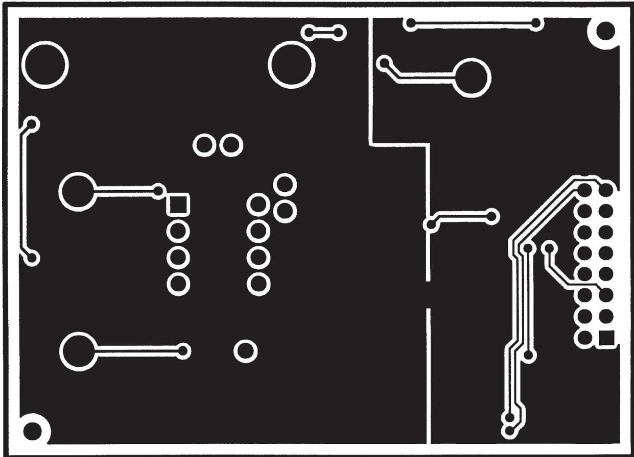
Figure 16d. Evaluation Circuit Board Solder Side Layout
