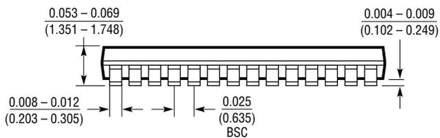
\* DIMENSION DOES NOT INCLUDE MOLD FLASH. MOLD FLASH SHALL NOT EXCEED 0.006" (0.152mm) PER SIDE
