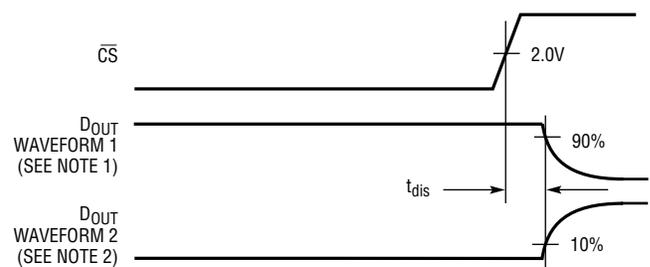
Voltage Waveform for  $D_{OUT}$  Delay Time,  $t_{dDO}$
