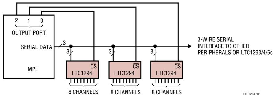
Figure 3. Several LTC1294 Sharing One 3-Wire Serial Interface
