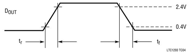
Voltage Waveform for  $t_{en\overline{SSO}}$
