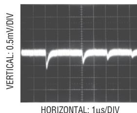
Figure 13. Adequate Reference Settling (LT1027)
