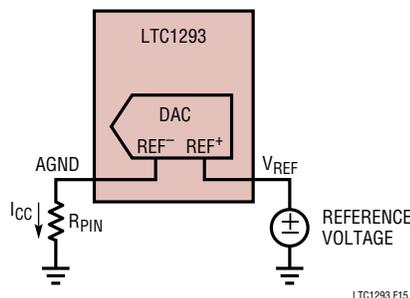
Figure 15. Parasitic Pin Resistance ( $R_{PIN}$ )
