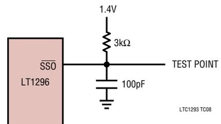
Load Circuit for  $t_{dis}$  and  $t_{en}$
