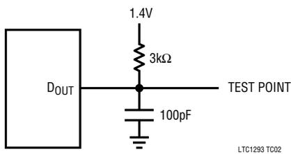
Load Circuit for  $t_{enSSO}$  and  $t_{disSSO}$
