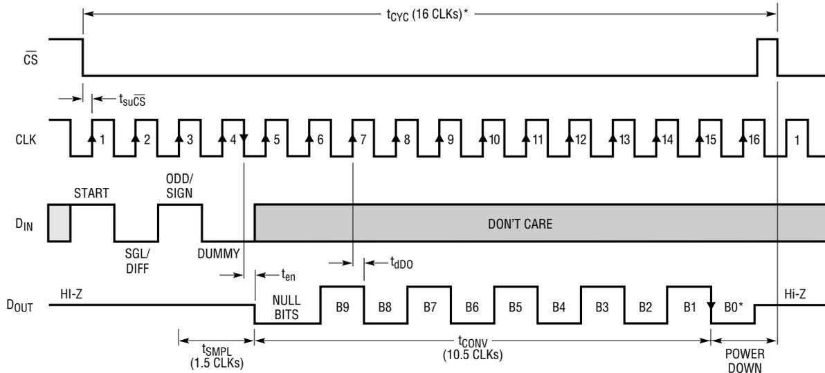
\*AFTER COMPLETING THE DATA TRANSFER, IF FURTHER CLOCKS ARE APPLIED WITH  $\overline{CS}$  LOW, THE ADC WILL OUTPUT ZEROS INDEFINITELY
