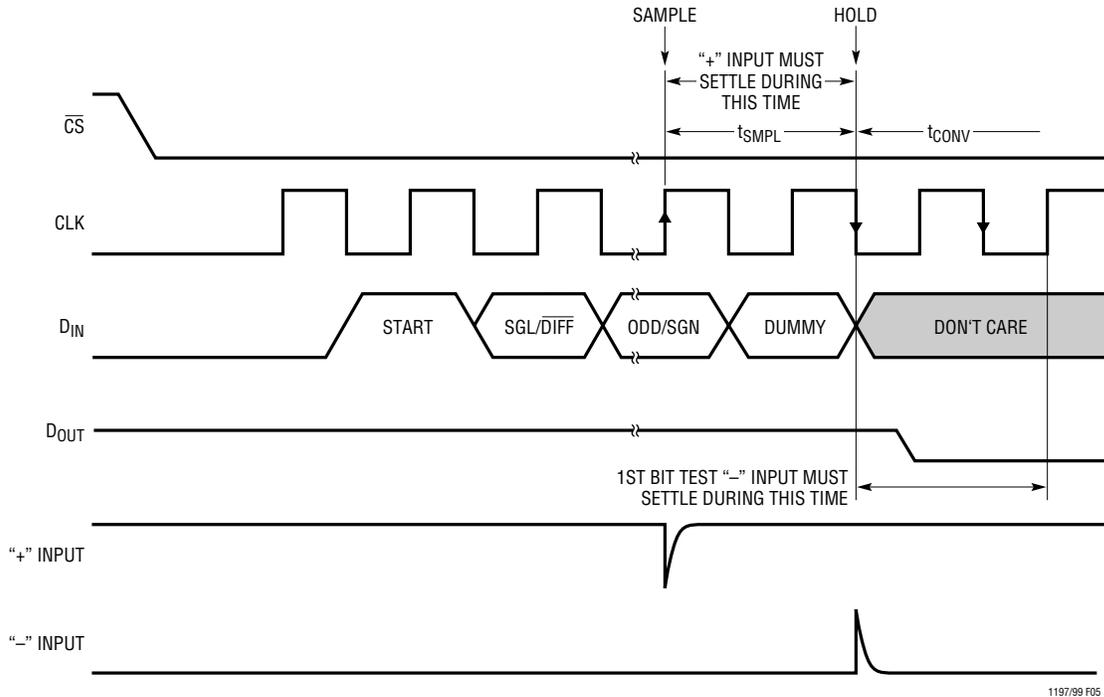
Figure 5. LTC1199/LTC1199L “+” and “-” Input Settling Windows
