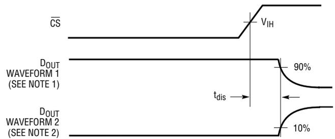
NOTE 1: WAVEFORM 1 IS FOR AN OUTPUT WITH INTERNAL CONDITIONS SUCH THAT THE OUTPUT IS HIGH UNLESS DISABLED BY THE OUTPUT CONTROL
