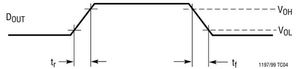
Voltage Waveforms for  $D_{OUT}$  Delay Time,  $t_{dDO}$
