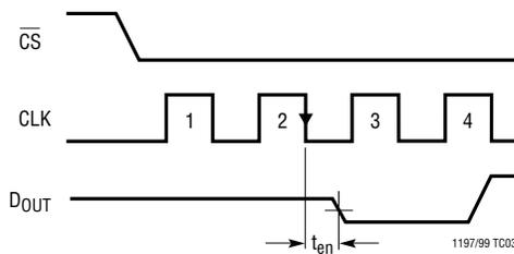
LTC1199/LTC1199L  $t_{en}$  Voltage Waveforms
