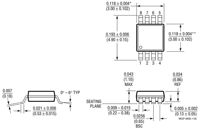
\* DIMENSION DOES NOT INCLUDE MOLD FLASH, PROTRUSIONS OR GATE BURRS. MOLD FLASH, PROTRUSIONS OR GATE BURRS SHALL NOT EXCEED  $0.006^*$  (0.152mm) PER SIDE
