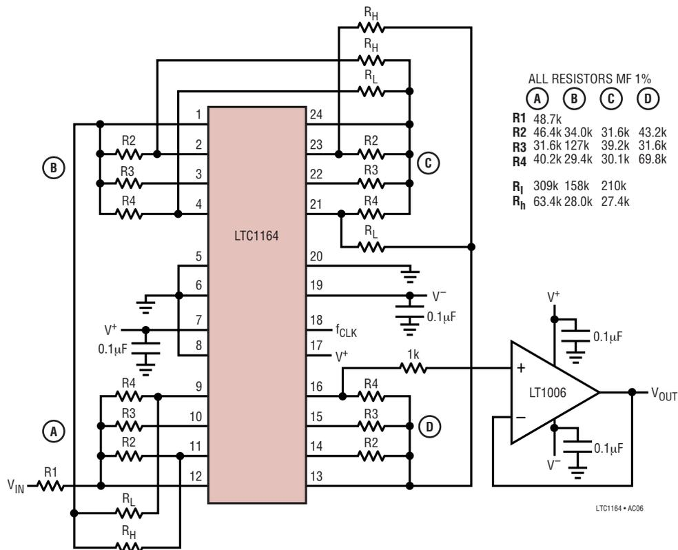
Figure 13. LTC1164 8th Order Lowpass Elliptic,  $f_{CUTOFF} = 5\text{kHz}$ ,  $f_{CLK} = 250\text{kHz}$ ,  $-78\text{dB}$  at  $10\text{kHz}$ , Passband Noise =  $110\mu\text{VRMS} \pm 5\text{V}$  (Also Refer to the LTC1164-6)
