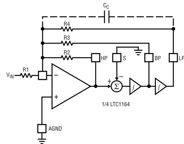
MODE 3 (100:1):  $f_o = \frac{f_{CLK}}{100} \sqrt{\frac{R_2}{R_4}}$ ;  $Q = \frac{R_3}{R_2} \sqrt{\frac{R_2}{R_4}}$ ;  $H_{OHP} = -R_2/R_1$ ;
