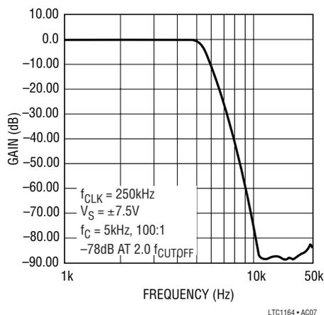
Figure 14. LTC1164 8th Order Lowpass Elliptic,  $f_{CUTOFF} = 5\text{kHz}$
