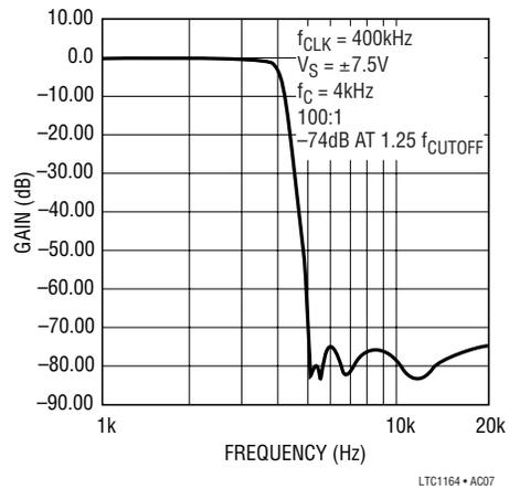
Figure 16. LTC1164 9th Order Lowpass Elliptic,  $f_{CUTOFF} = 4\text{kHz}$
