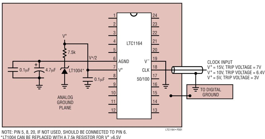
Figure 2. Single Supply Operation
