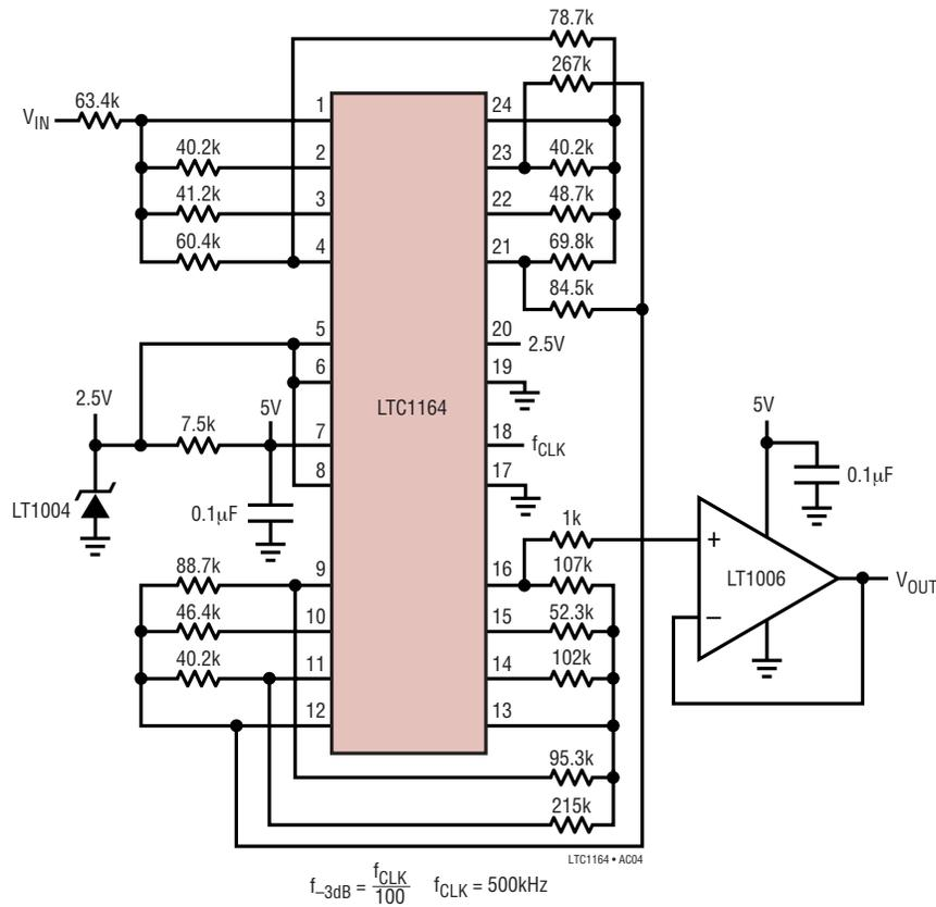
Figure 12. 8th Order Lowpass Single Supply Elliptic-Bessel Transitional Filter
