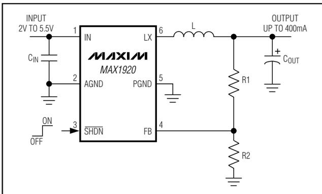
Figure 4. MAX1920 Application Circuit Using Tantalum Output Capacitor
