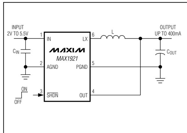
Figure 3. MAX1921 Application Circuit Using Tantalum Output Capacitor
