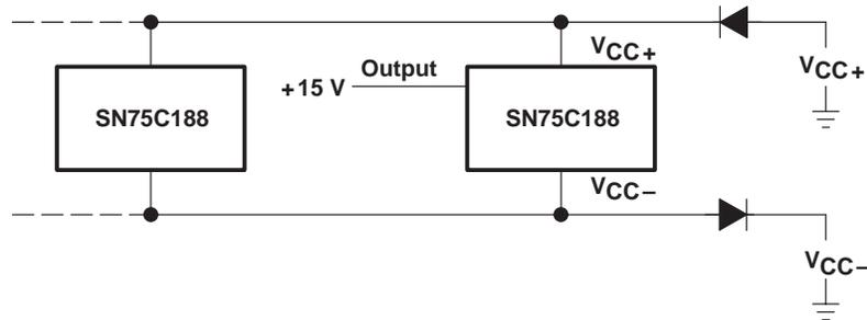
NOTE A: External diodes placed in series with the  $V_{CC+}$  and  $V_{CC-}$  leads protect the SN75C188 in the fault condition where the device outputs are shorted to  $\pm 15$  V and the power supplies are at low voltage and provide low-impedance paths to GND.
