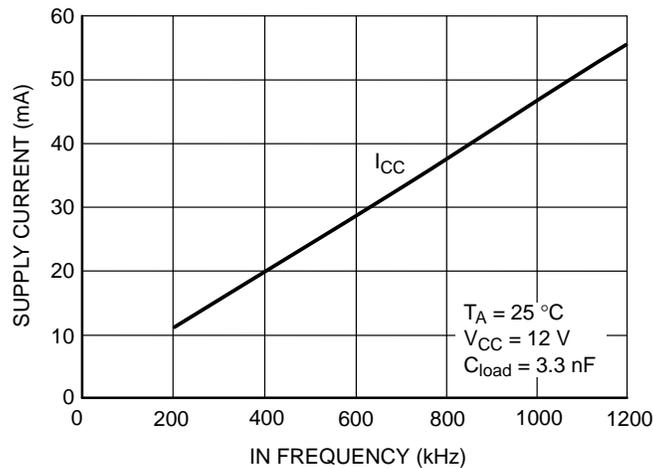
Figure 8.  $V_{CC}$  Supply Current vs. IN Frequency
