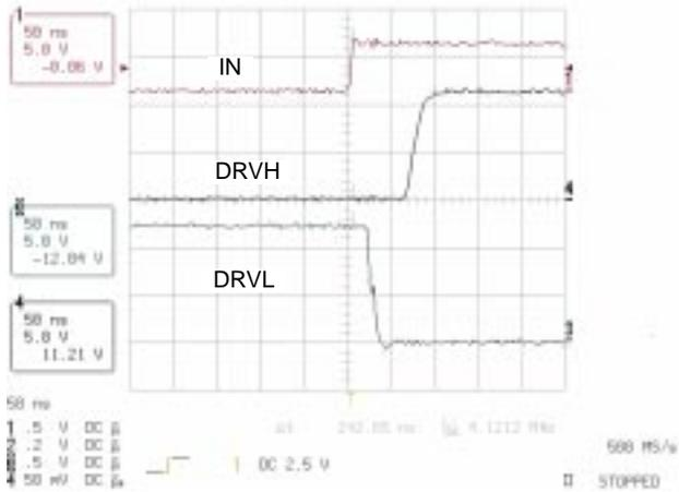
Figure 4. DRVH Rise and DRVL Fall Times
