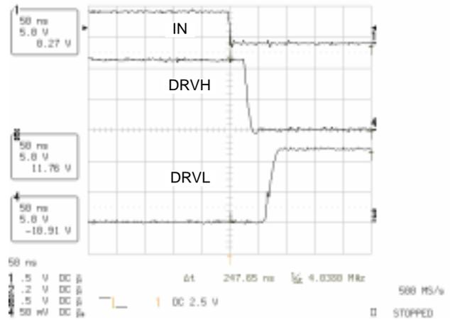
Figure 5. DRVH Fall and DRVL Rise Times
