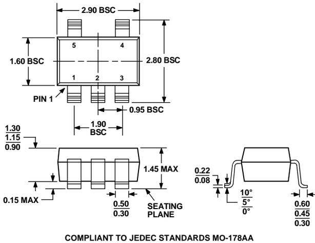
Figure 66. 5-Lead Small Outline Transistor Package [SOT-23] (RT-5)
