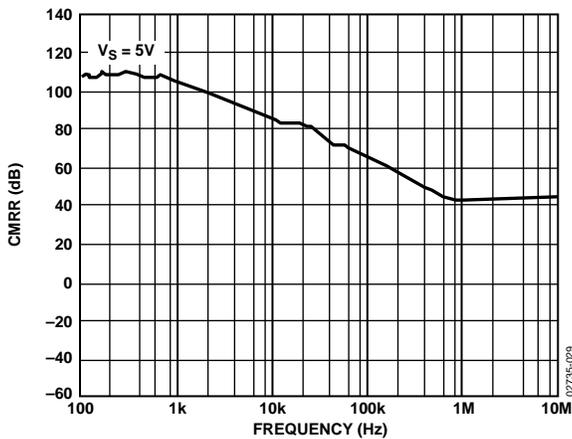
Figure 31. CMRR vs. Frequency at 5 V
