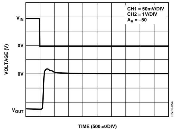
Figure 57. Positive Input Overload Recovery for LTC2050
