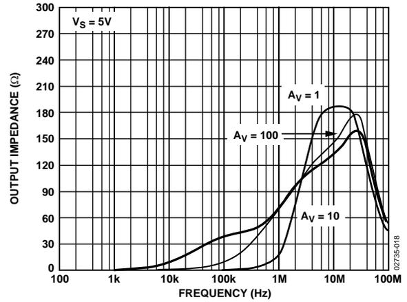
Figure 20. Output Impedance vs. Frequency at 5 V
