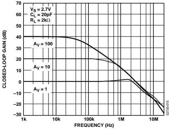
Figure 17. Closed-Loop Gain vs. Frequency at 2.7 V
