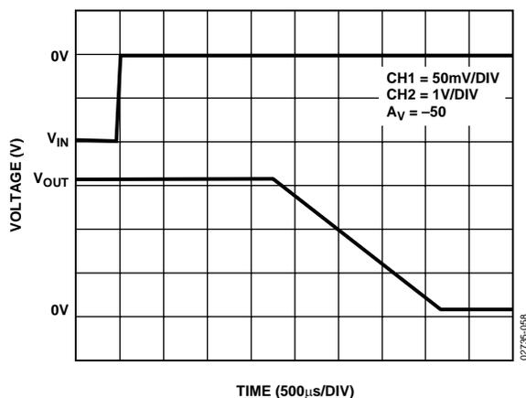
Figure 61. Negative Input Overload Recovery for LMC2001
