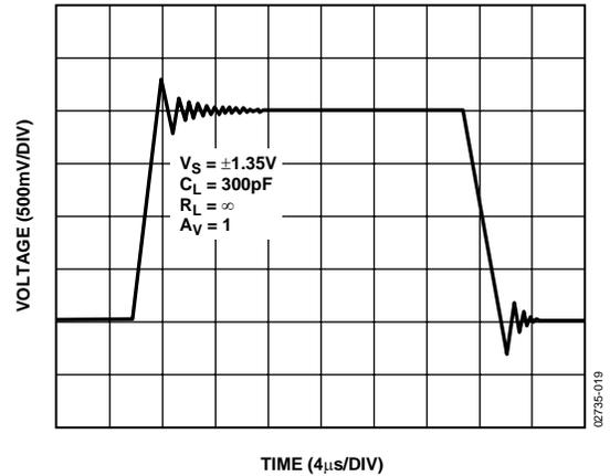
Figure 21. Large Signal Transient Response at 2.7 V
