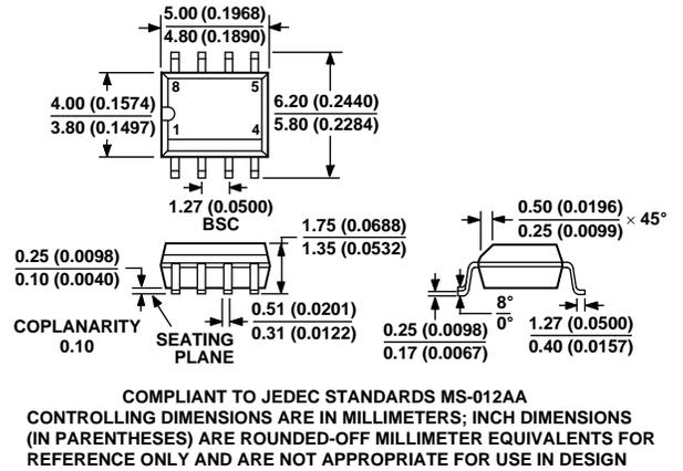
Figure 67. 8-Lead Standard Small Outline Package [SOIC] Narrow Body (R-8)
