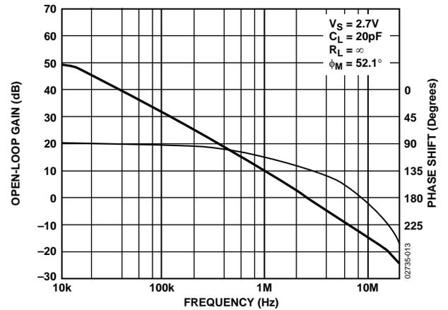
Figure 15. Open-Loop Gain and Phase vs. Frequency
