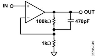
Figure 52. Test Circuit: First-Order Low-Pass Filter—×101 Gain and 3 kHz Corner Frequency
