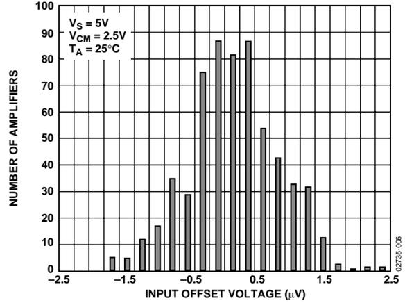
Figure 8. Input Offset Voltage Distribution at 5 V
