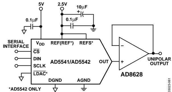
Figure 64. AD8628 Used as an Output Amplifier
