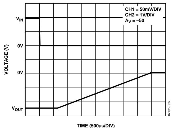
Figure 58. Positive Input Overload Recovery for LMC2001
