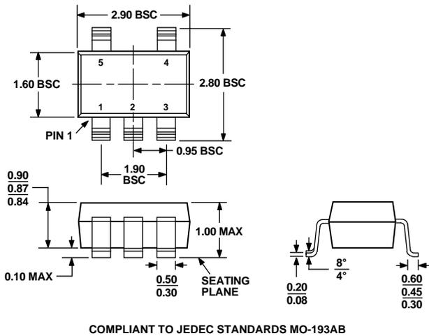
Figure 65. 5-Lead Thin Small Outline Transistor Package [TSOT] (UJ-5)
