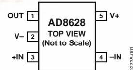
Figure 1. 5-Lead TSOT (UJ-5) and 5-Lead SOT-23 (RT-5)
