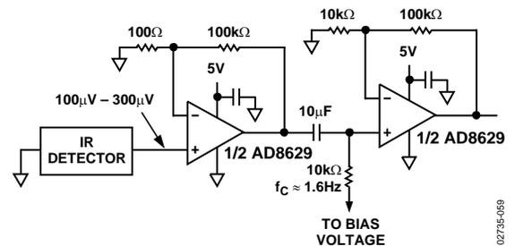
Figure 62. AD8629 Used as Preamplifier for Thermopile
