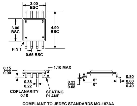
Figure 65. 8-Lead Standard Small Outline Package [MSOP] (RM-8)
