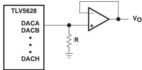
NOTE A: Resistor  $R \geq 10 \text{ k}\Omega$
