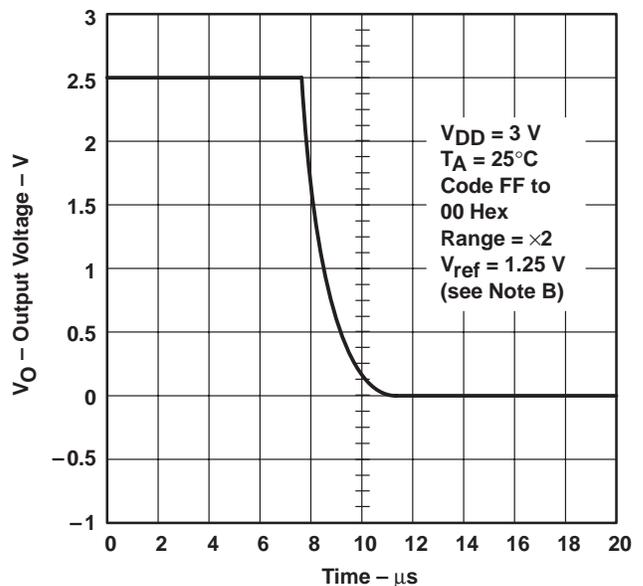
NOTE B: Fall time = 4.25  $\mu$ s, negative slew rate = 0.46 V/ $\mu$ s, settling time = 8.5  $\mu$ s.
