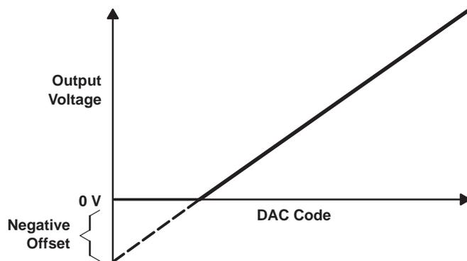
Figure 5. Effect of Negative Offset (Single Supply)
