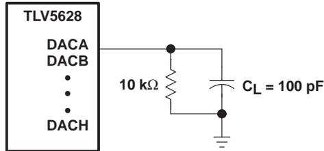
Figure 6. Slewing Settling Time and Linearity Measurements
