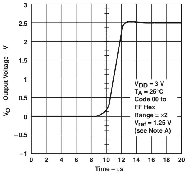
NOTE A: Rise time = 2.05  $\mu$ s, positive slew rate = 0.96 V/ $\mu$ s, settling time = 4.5  $\mu$ s.
