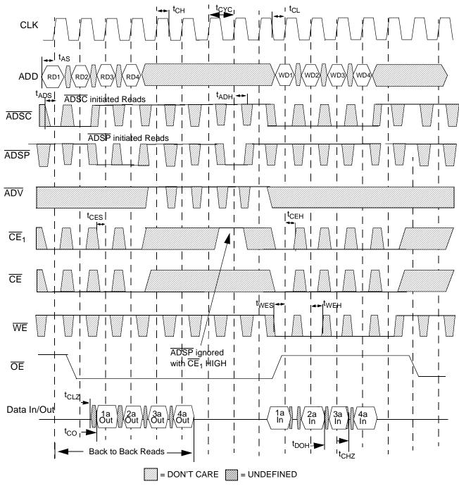
Device originally deselected.  $\overline{\text{CE}}$  is the combination of  $\overline{\text{CE}}_2$  and  $\overline{\overline{\text{CE}}}_3$ . All chip selects need to be active in order to select the device.
