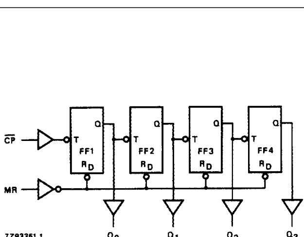
Fig.6 Logic diagram (one counter).
