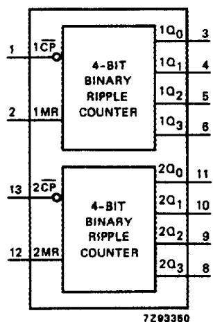
Fig.4 Functional diagram.
