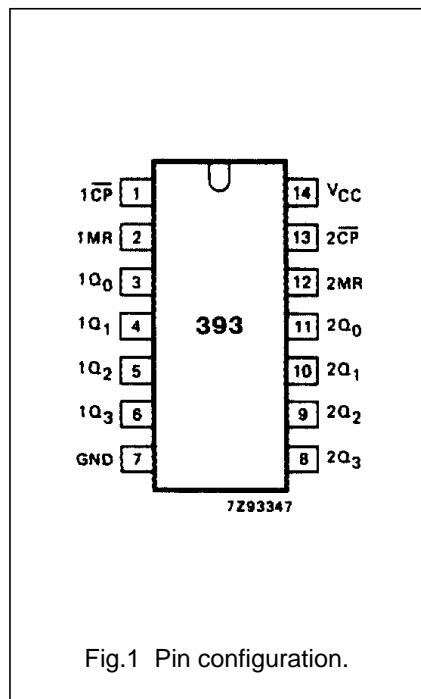
Fig.1 Pin configuration.
