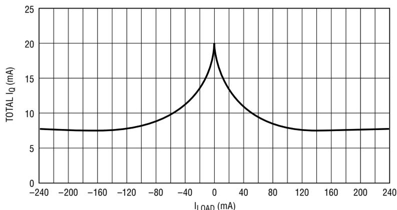
Figure 7. I<sub>Q</sub> vs I<sub>LOAD</sub>
