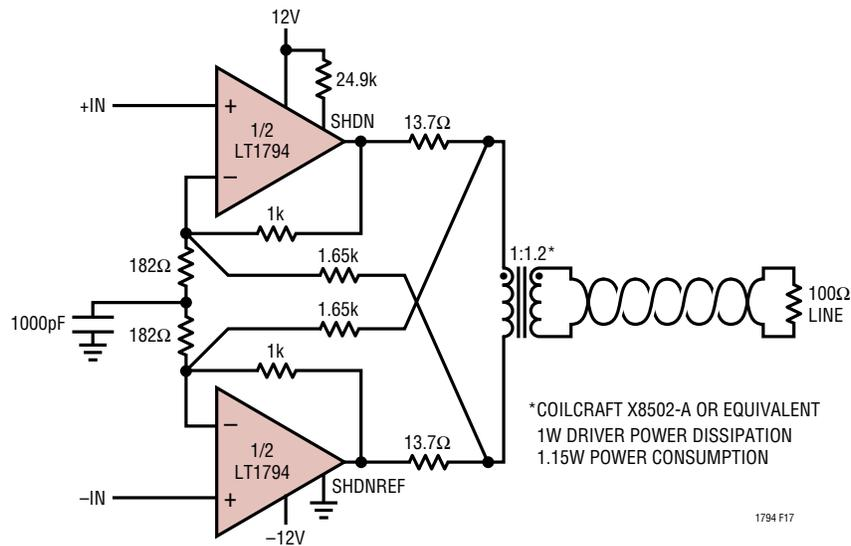
**Figure 17. ADSL Line Driver Using Active Termination**
