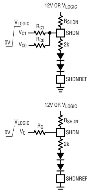
Figure 4. Providing Logic Input Control of Operating Current
