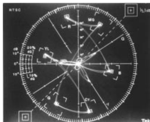
Vector Plot of Standard Color Burst Through 1000 Feet of Twisted-Pair
