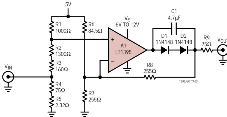
Figure 3. Single Supply RGB Video Amplifier (1 of 4 Channels)
