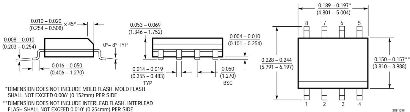
\*DIMENSION DOES NOT INCLUDE MOLD FLASH. MOLD FLASH SHALL NOT EXCEED  $0.006^*$  (0.152mm) PER SIDE
