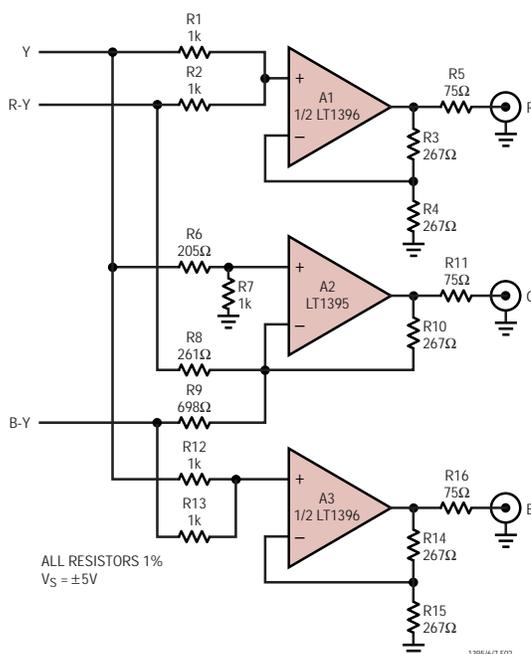
Figure 2. Buffered Color-Difference to RGB Matrix
