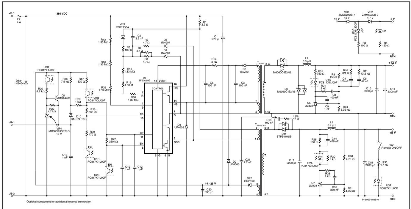
Figure 27. Schematic of High-Efficiency +12 V, 25 A Main Output and +5 V, 2.5 A Standby Power Supply.
