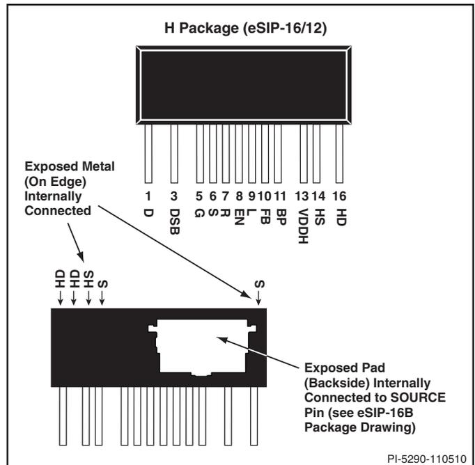
Figure 2. Pin Configuration.
