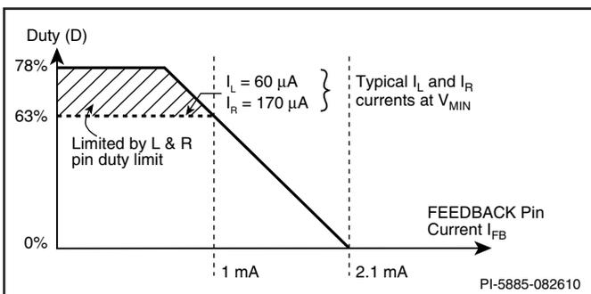
Figure 7. PWM Duty Cycle vs. Control Current.
