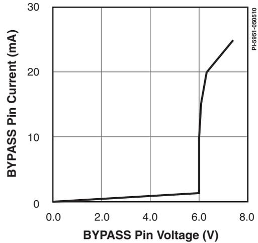
Figure 40. BYPASS Pin Current vs. BYPASS Pin Voltage.
