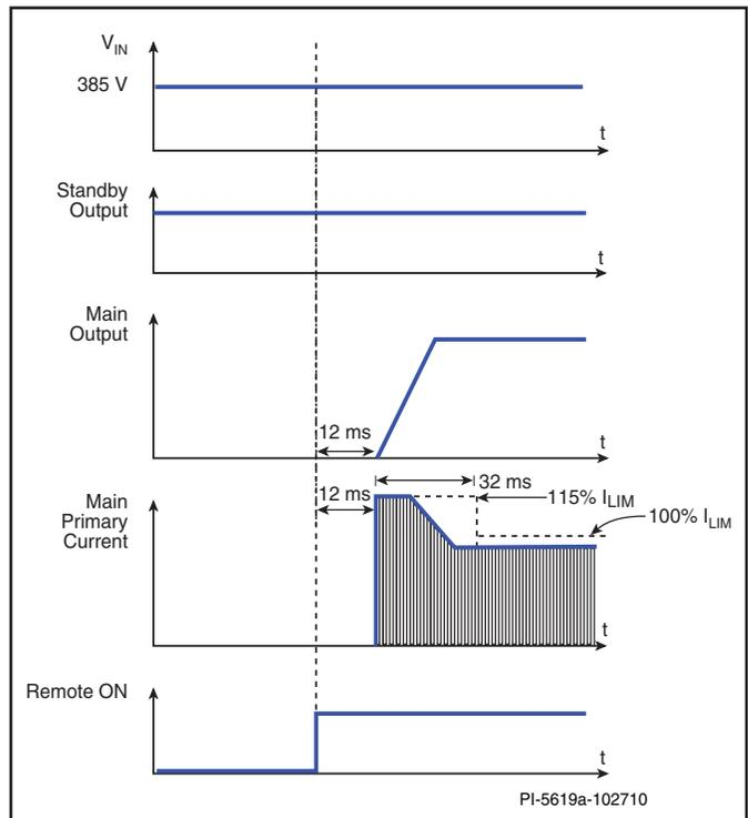
Figure 6. Supply Start-Up Sequence by Remote ON.
