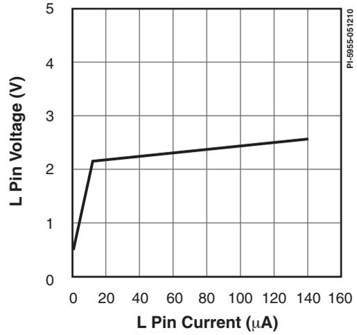
Figure 36. L Pin Voltage vs. L Pin Current.
