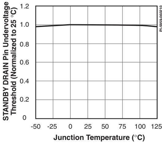
Figure 35. Standby Supply, Undervoltage Threshold vs. Junction Temperature.
