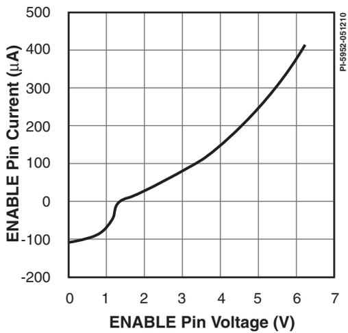
Figure 39. ENABLE Pin Current vs. ENABLE Pin Voltage.
