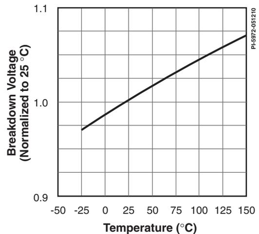
Figure 52. High-Side MOSFET Breakdown Voltage vs. Temperature.
