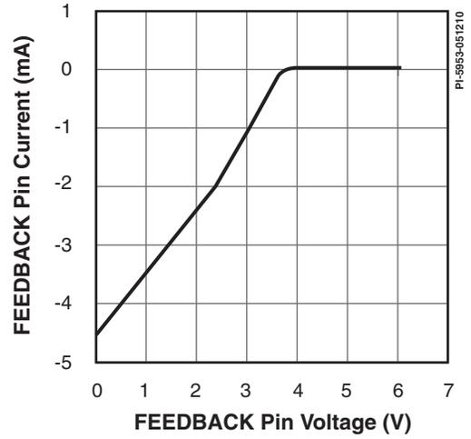
Figure 38. FEEDBACK Pin Current vs. FEEDBACK Pin Voltage.
