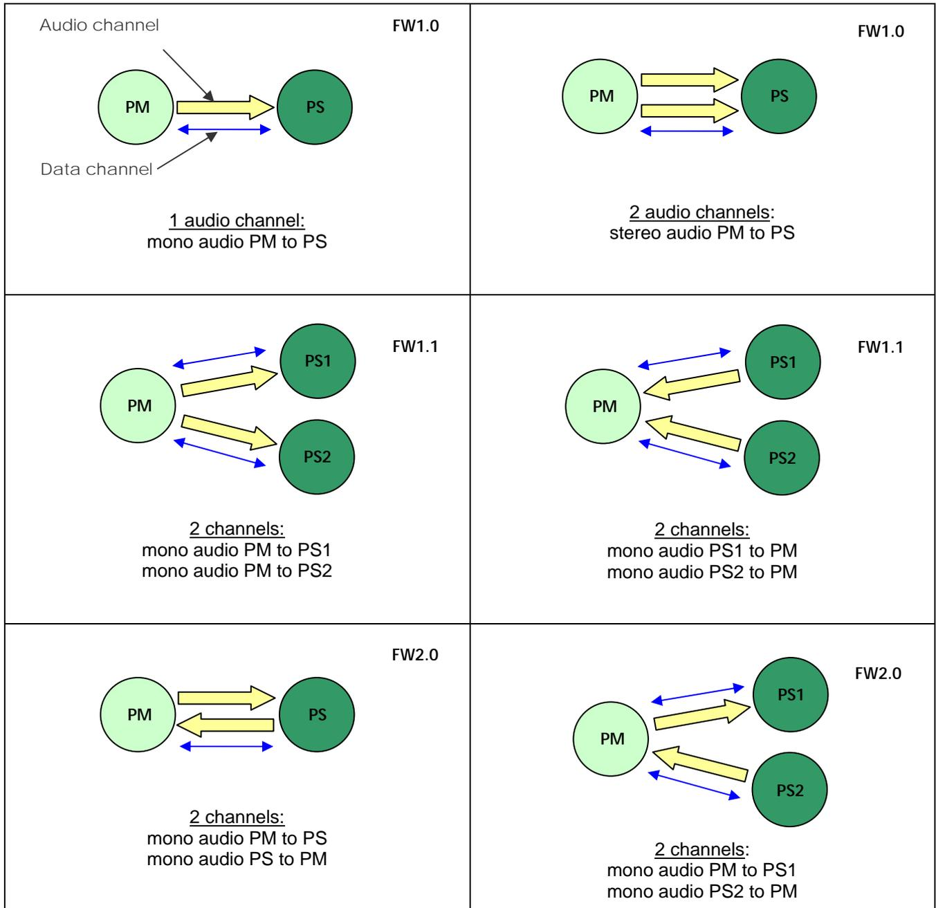
**Figure 3 CC8520 topologies supported for different CC8520 FW revisions**
