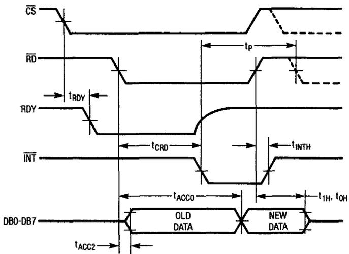
Figure 2. RD Mode (Pin 7 is GND)
