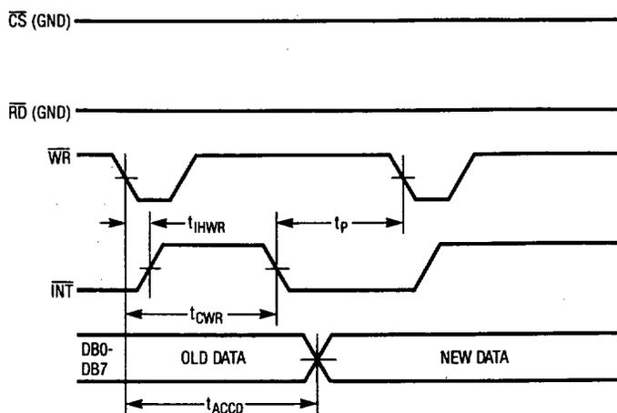
Figure 4. WR-RD Mode (Pin 7 is HIGH) Stand-Alone Operation
