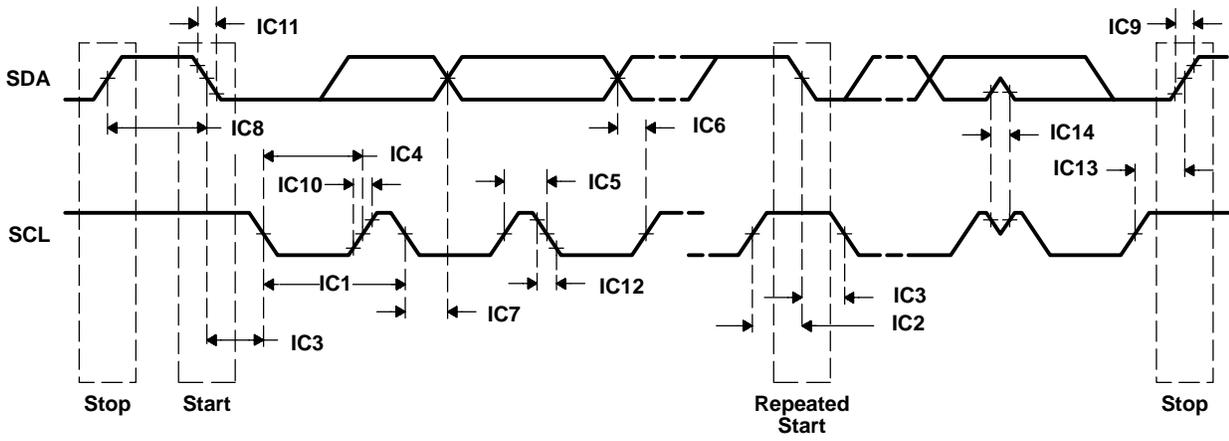
Figure 5-37. I<sup>2</sup>C Receive Timings
