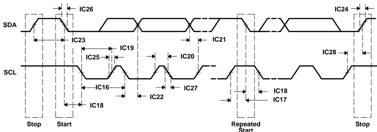
Figure 5–38. I<sup>2</sup>C Transmit Timings
