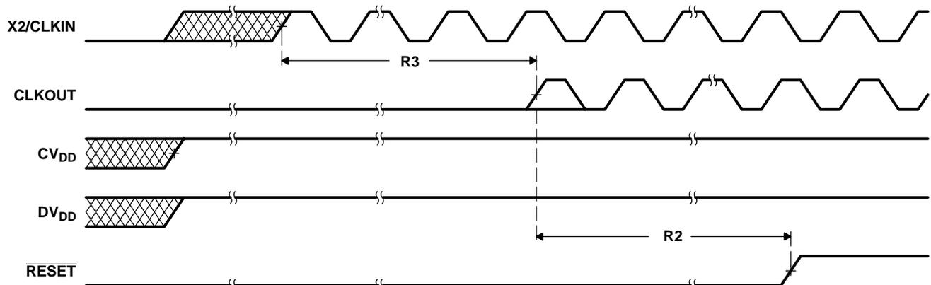
**Figure 5–16. Power-Up Reset (On-Chip Oscillator Inactive) Timings**
