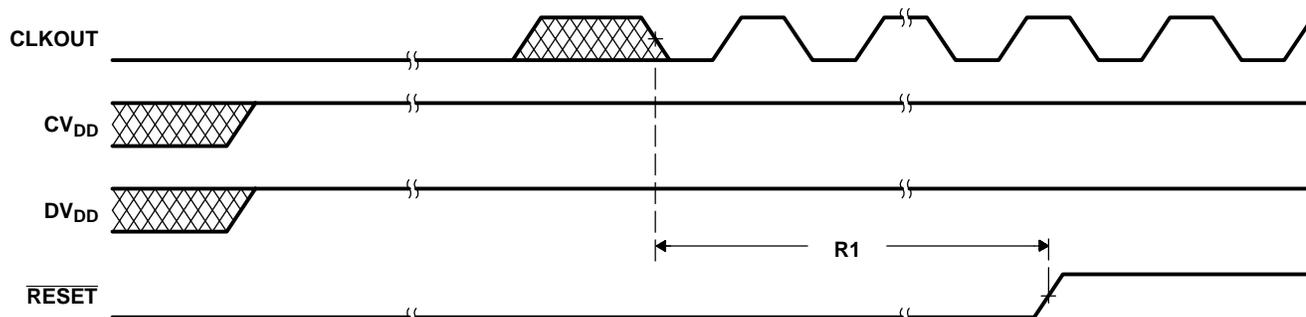
**Figure 5–15. Power-Up Reset (On-Chip Oscillator Active) Timings**
