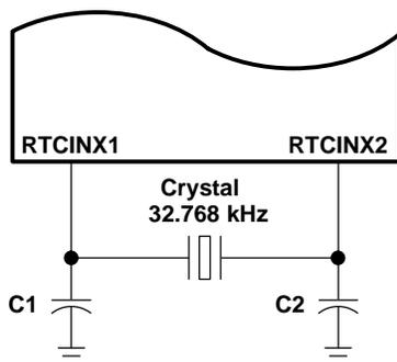
Figure 5–5. Real-Time Clock Oscillator With External Crystal
