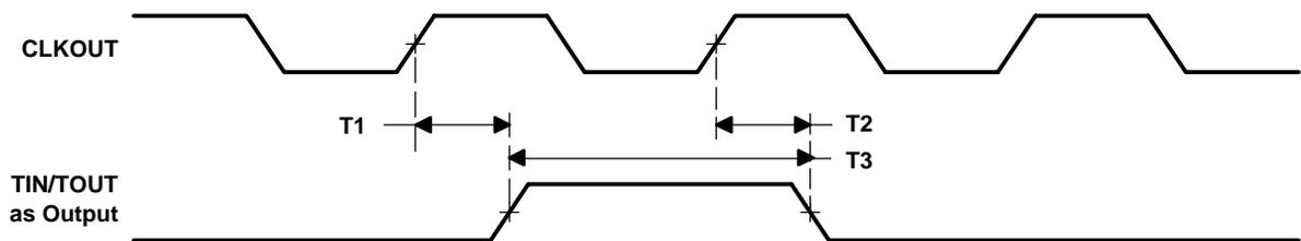
**Figure 5–23. TIN/TOUT Timings When Configured as Outputs**
