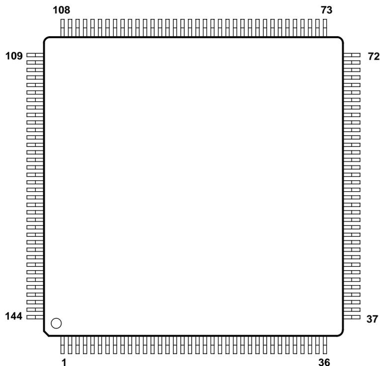
Figure 2–2. 144-Pin PGE Low-Profile Quad Flatpack (Top View)
