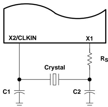
Figure 5–2. Internal System Oscillator With External Crystal
