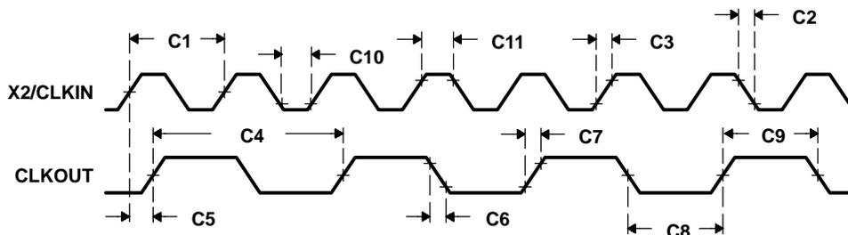
NOTE A: The relationship of X2/CLKIN to CLKOUT depends on the PLL bypass divide factor chosen for the CLKMD register. The waveform relationship shown in Figure 5–3 is intended to illustrate the timing parameters based on CLKOUT = 1/2(CLKIN) configuration.
