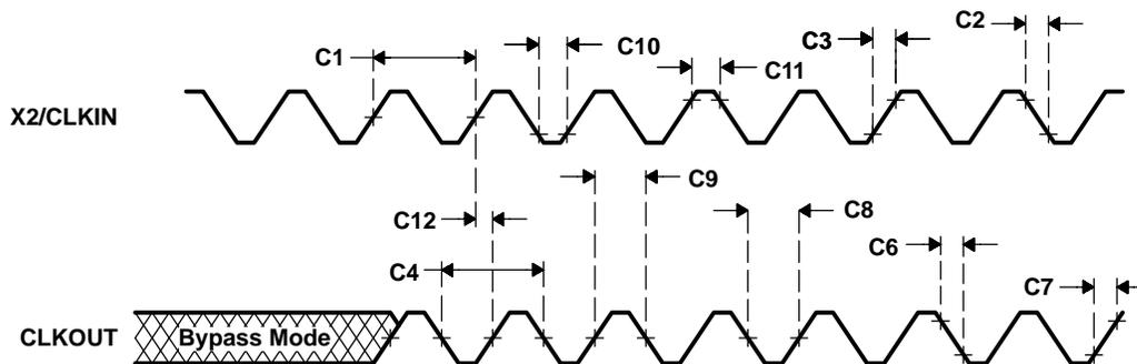
NOTE A: The relationship of X2/CLKIN to CLKOUT depends on the PLL multiply and divide factor chosen for the CLKMD register. The waveform relationship shown in Figure 5–3 is intended to illustrate the timing parameters based on CLKOUT = 1xCLKIN configuration.
