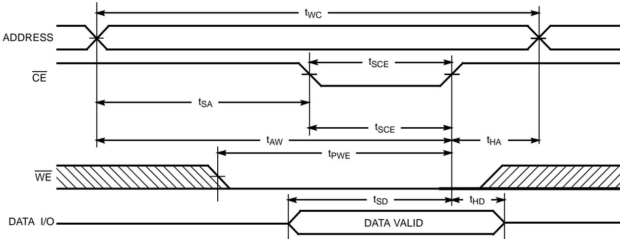
**Write Cycle No. 2 ( $\overline{WE}$  Controlled,  $\overline{OE}$  HIGH During Write)<sup>[15, 16]</sup>**
