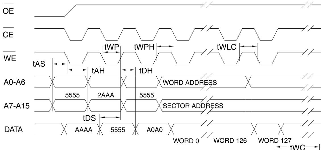
1. A7 through A15 must specify the same page address during each high to low transition of WE (or CE) after the software code has been entered.
