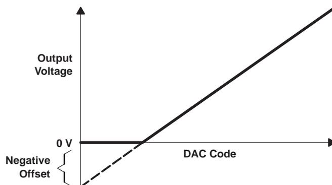
Figure 10. Effect of Negative Offset (Single Supply)
